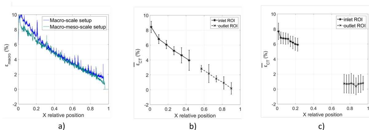
Figure I.46: Macroscopic decompaction evaluation: a) using the *Macro-scale* methodology (confocal chromatic scanner). b) using the *Macro-meso-scale* methodology (CT-scan) and the *Macro-meso-scale* setup. c) using the *Meso-scale* methodology (CT-scan) and the *Meso-scale* setup.
