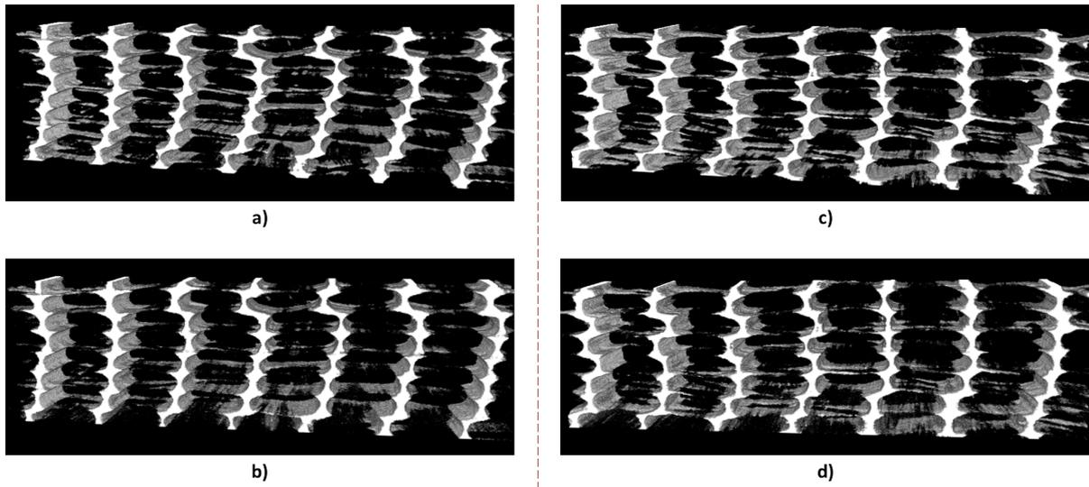
Figure I.39: 3D visualization of the inter-tow channels (threshold=155): a) inlet ROI (centered around  $X=0.1$ ), dry state. b) inlet ROI (centered around  $X=0.1$ ), saturated state. c) outlet ROI (centered around  $X=0.8$ ), dry state. d) outlet ROI (centered around  $X=0.8$ ), saturated state.
