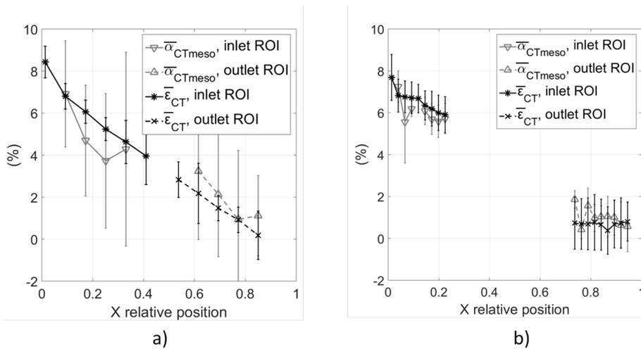
Figure I.49: Computation of the macroscopic decompaction (vertical vacuum bag displacement  $\bar{\epsilon}_{CT}$ ) and the mesoscopic decompaction (tows area evolution  $\bar{\alpha}_{CTmeso}$ ): a) results obtained with the *Macro-meso-scale* approach. b) results obtained with the *Meso-scale* approach.
