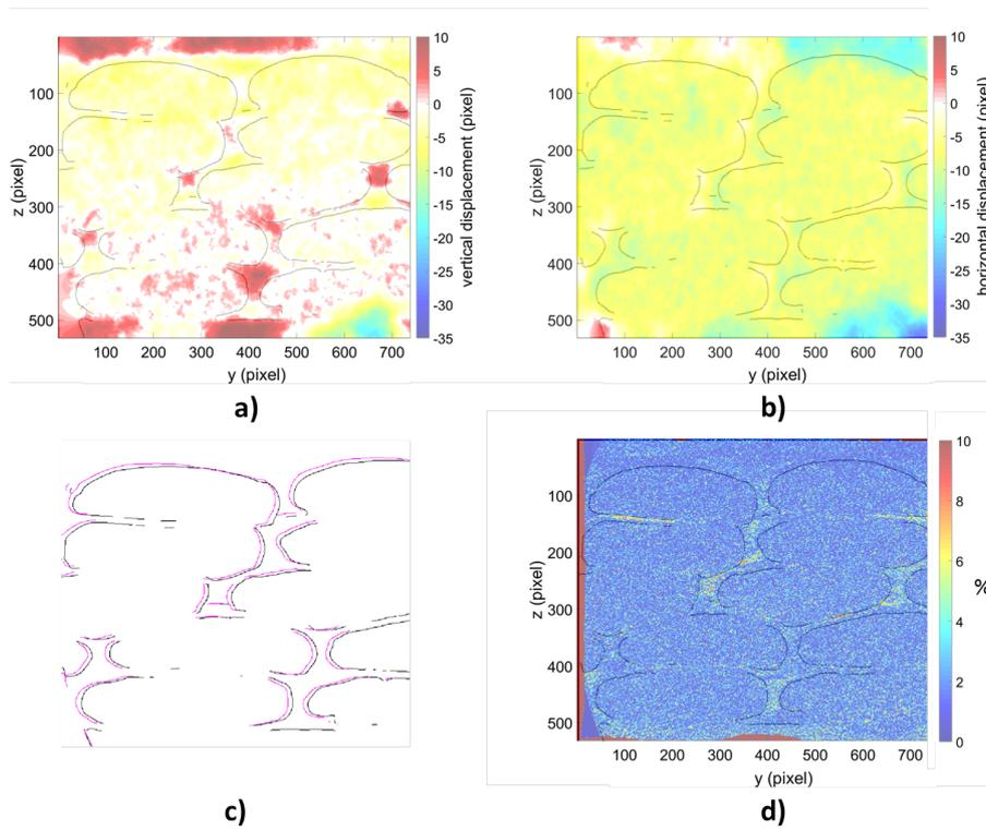
Figure I.48: Displacement fields between the dry and the saturated states at an X-position near the vacuum vent ( $X=0.76$ ): a) Vertical microstructure displacement (Z-axis) in voxel. b) Horizontal microstructure displacement (Y-axis) in voxel. c) Visualization of the microstructure evolution (in black: dry state, in pink: saturated state. d) Error of the Thirion algorithm for the considered images.
