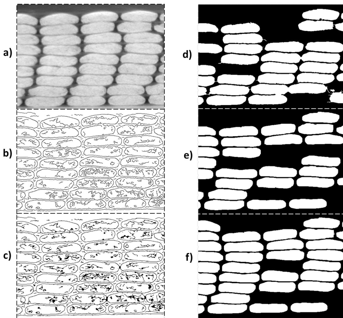
Figure I.33: Illustration of the post-processing for a concatenated slice centered near the fluid inlet ( $X=0.01$ , e.g.  $x=0.9$  mm). a) Concatened slice (raw). b) Application of Canny edge detection and threshold. c) Closing the boundaries. d) Filling of the tows and cleaning. e) Erosion of the burrs. f) Addition of the tows detected on the corresponding 150-slices-concatened image.
