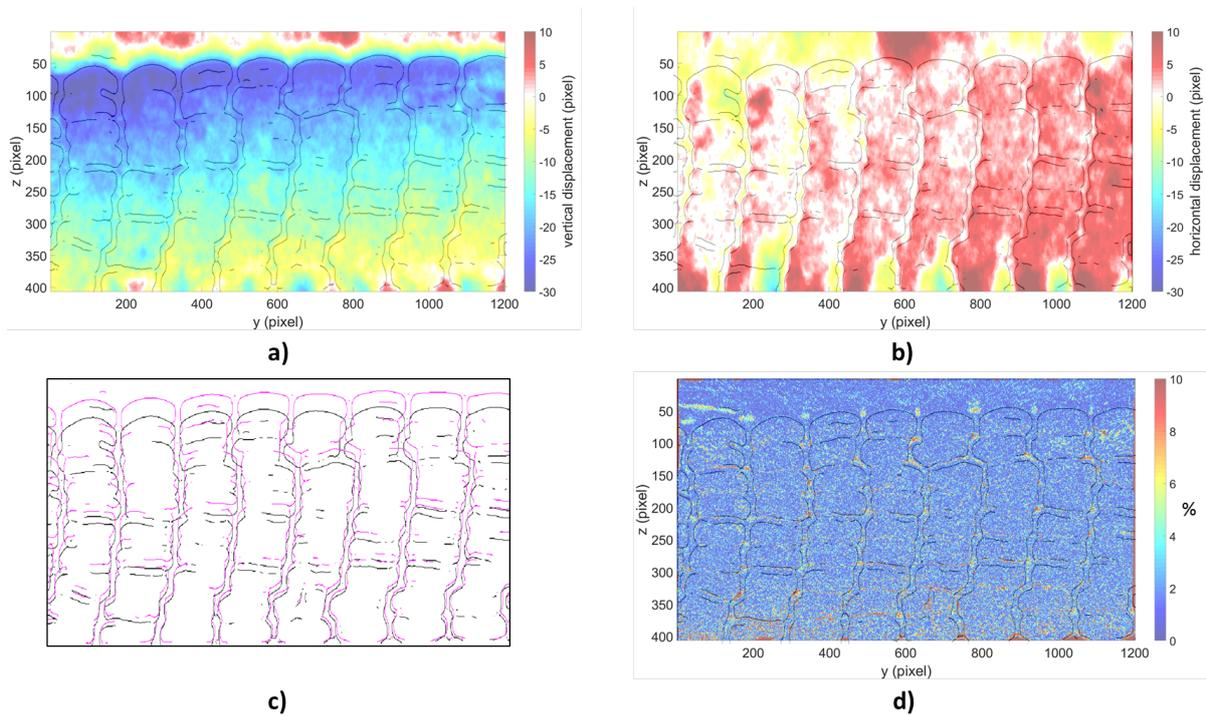
Figure I.36: Displacement fields between the dry and the saturated states at an X-position near the fluid inlet ( $X=0.1$ ): a) Vertical microstructure displacement (Z-axis) in voxel. b) Horizontal microstructure displacement (Y-axis) in voxel. c) Visualization of the microstructure evolution (in black: dry state, in pink: saturated state). d) Error of the Thirion algorithm for the considered images.
