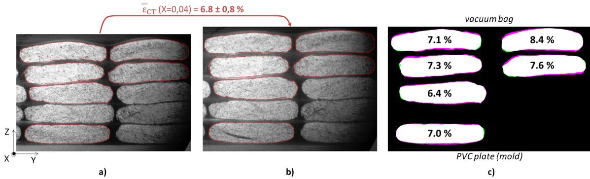
Figure I.51: Illustration and quantification of tow deformation near the inlet ( $X=0.04$ ):
