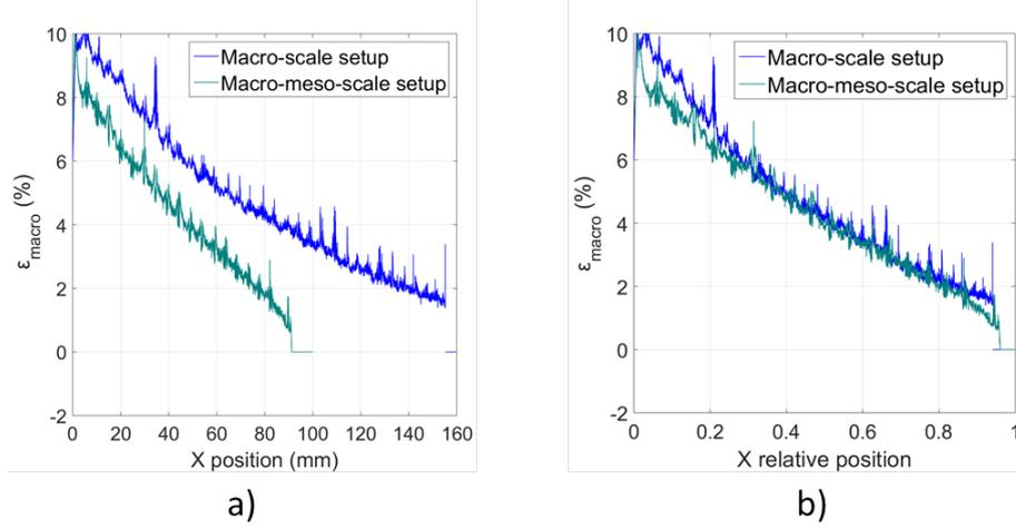
Figure I.23: Comparison of the decompaction gradient obtained with the *Macro-* and the *Macro-meso scale* setups: a) representation with the real flow length. b) adimensionalization of the flow length.
