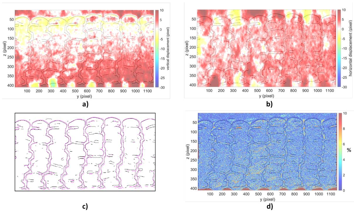
Figure I.37: Displacement fields between the dry and the saturated states at an X-position near the vacuum vent ( $X=0.8$ ): a) Vertical microstructure displacement (Z-axis) in voxel. b) Horizontal microstructure displacement (Y-axis) in voxel. c) Visualization of the microstructure evolution (in black: dry state, in pink: saturated state). d) Error of the Thirion algorithm for the considered images.
