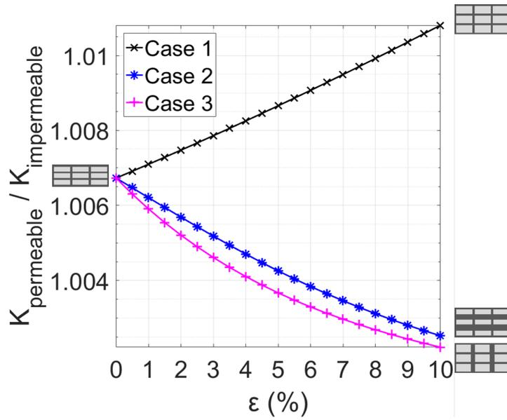
Figure I.55: Ratio  $\frac{K_{permeable}}{K_{impermeable}}$  evolution with stack thickness rise for the 3 proposed microstructural reorganizations
