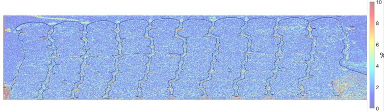
Figure I.31: Error computed between the dry state (R) and the deformed saturated state (D) near the inlet ( $X=0.08$ ). To enhance the interpretation, the partial detected tows boundaries are also reported.
