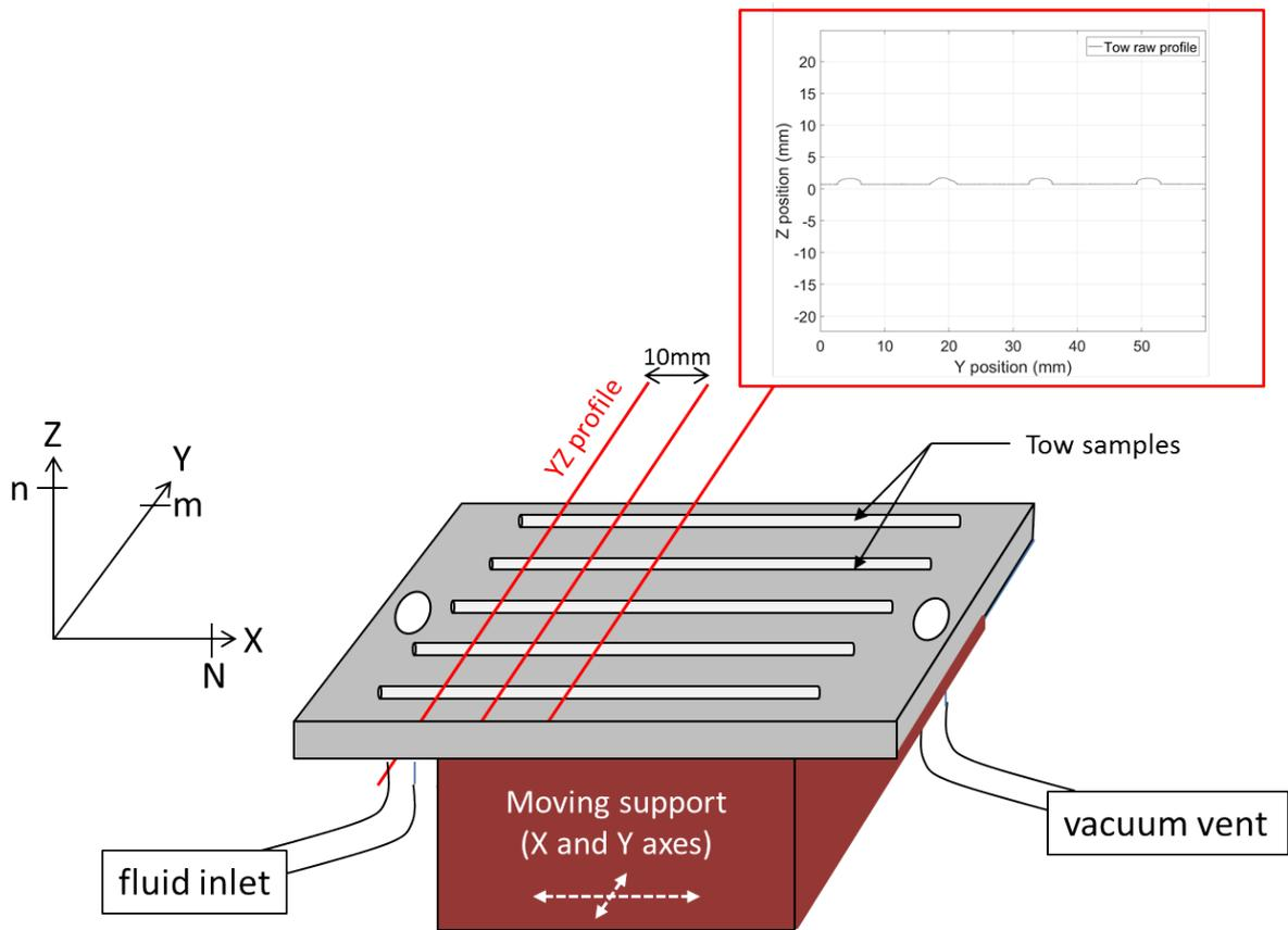
Figure III.2: Schematic view of the overall setup placed on the CCS moving support. Precisions about the recorded data are given  $(N, m, n)$ .
