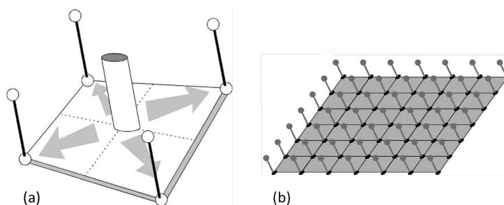
Figure II.3: 1D "slave" element attached to all the nodes of a "master" element [54]:
