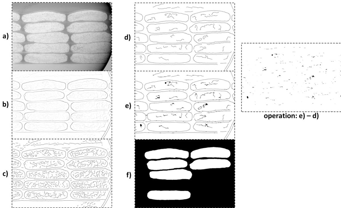
Figure I.43: Illustration of the post-processing for a concatenated slice centered near the fluid inlet ( $x=3\text{mm}$ ). a) Concatenated slice (raw). b) Application of FeatureJ. c) Selection of the significant edges by thresholding. d) Application of a minimum connected black pixels. e) Boundaries closing (an operation is presented to enhance the visibility "e)-d)"). f) Filled tows.
