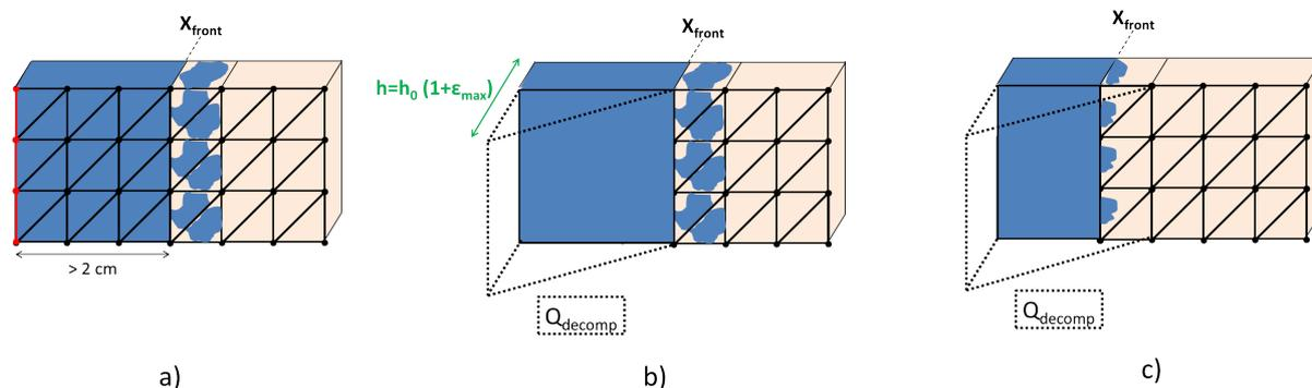
Figure II.9: Illustration of the methodology to ensure mass balance: a) time step  $n$ , before introducing the decompaction. b) time step  $n$ , after introducing decompaction, before the emptying phase. c) time step  $n$ , after the emptying phase.  $X_{front}$  is the fully saturated flow front position.
