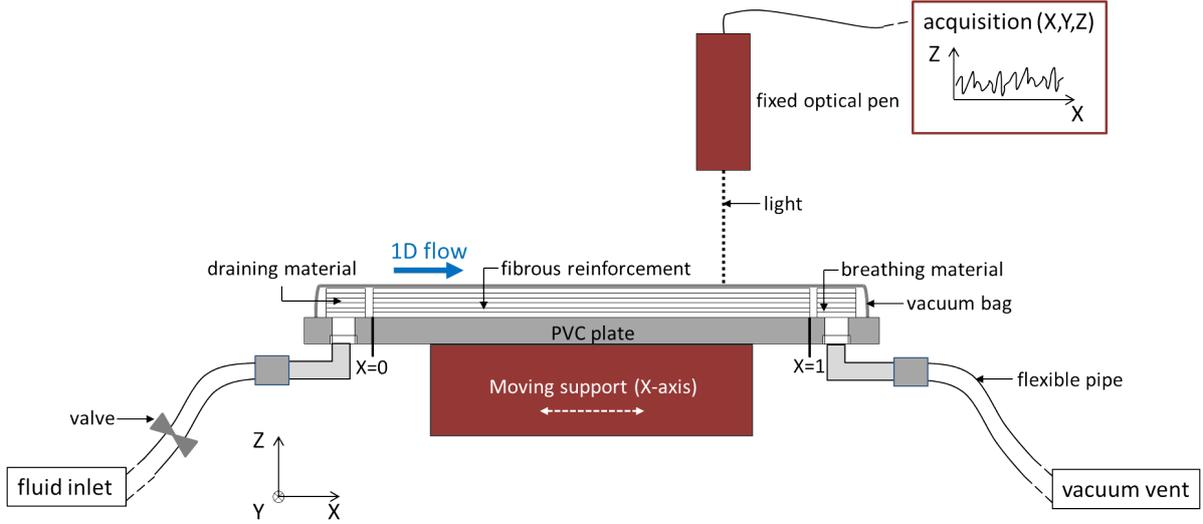
Figure I.5: Schematic view of the *Macro-scale* setup: acquisition equipment (in red) and infusion setup (in grey)
