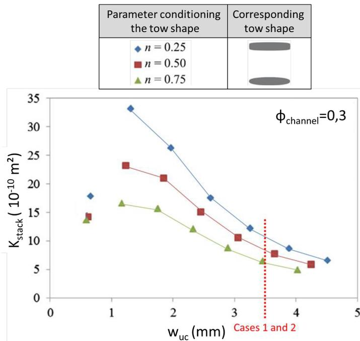
Figure I.56: Evolution of the in-plane permeability for several tow cross-sectional shapes, at a given channel content ( $\phi_{channels}=0.3$ ) [35]
