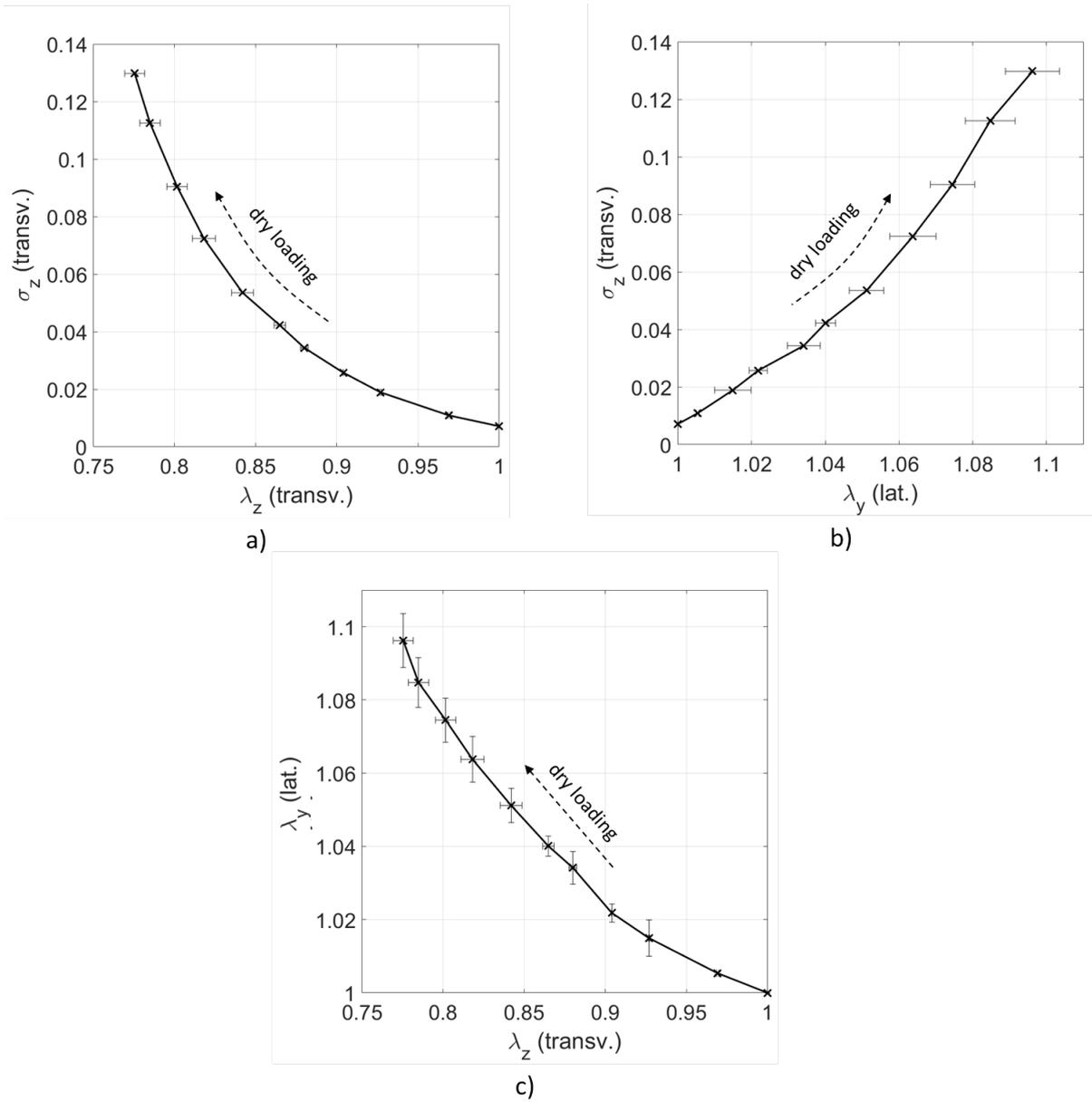
Figure III.18: Single tow evolution during the dry unidirectional loading stage: a) transverse strain extension with stress. b) lateral strain extension with stress. c) transverse strain extension with lateral strain extension.
