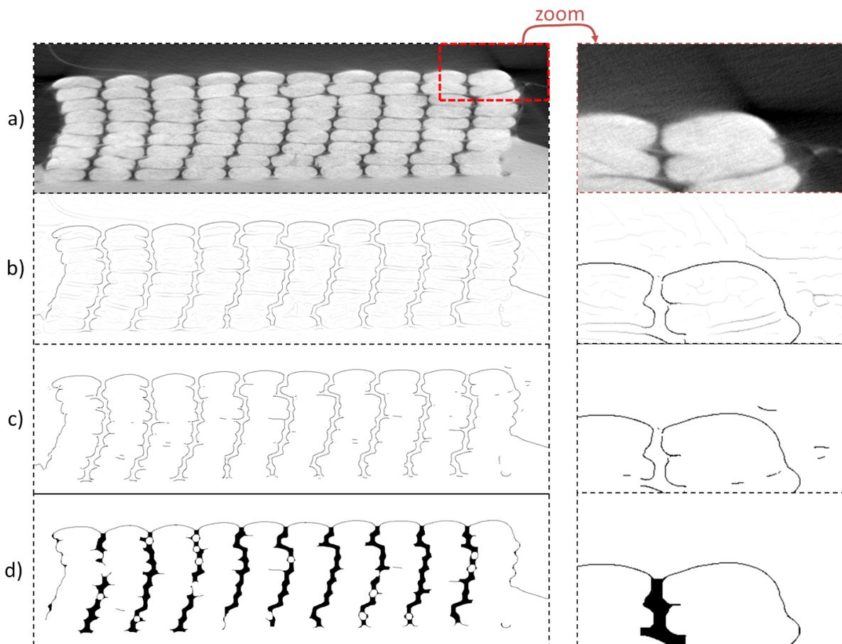
Figure I.20: Illustration of the post-processing on a slice selected near the fluid inlet ( $X=0.09$ ). a) Raw image after the cropping step. b) Application of the FeatureJ plugin. c) Selection of the significant edges. d) Remove of the isolated black pixels and horizontal closing of the gap between upper tows.
