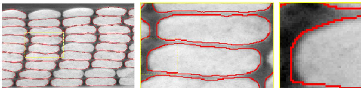
Figure I.34: Superposition of a 100-slices-concatened image and the corresponding detected tow boundaries. Several zoomed views are presented to enhance the analysis.
