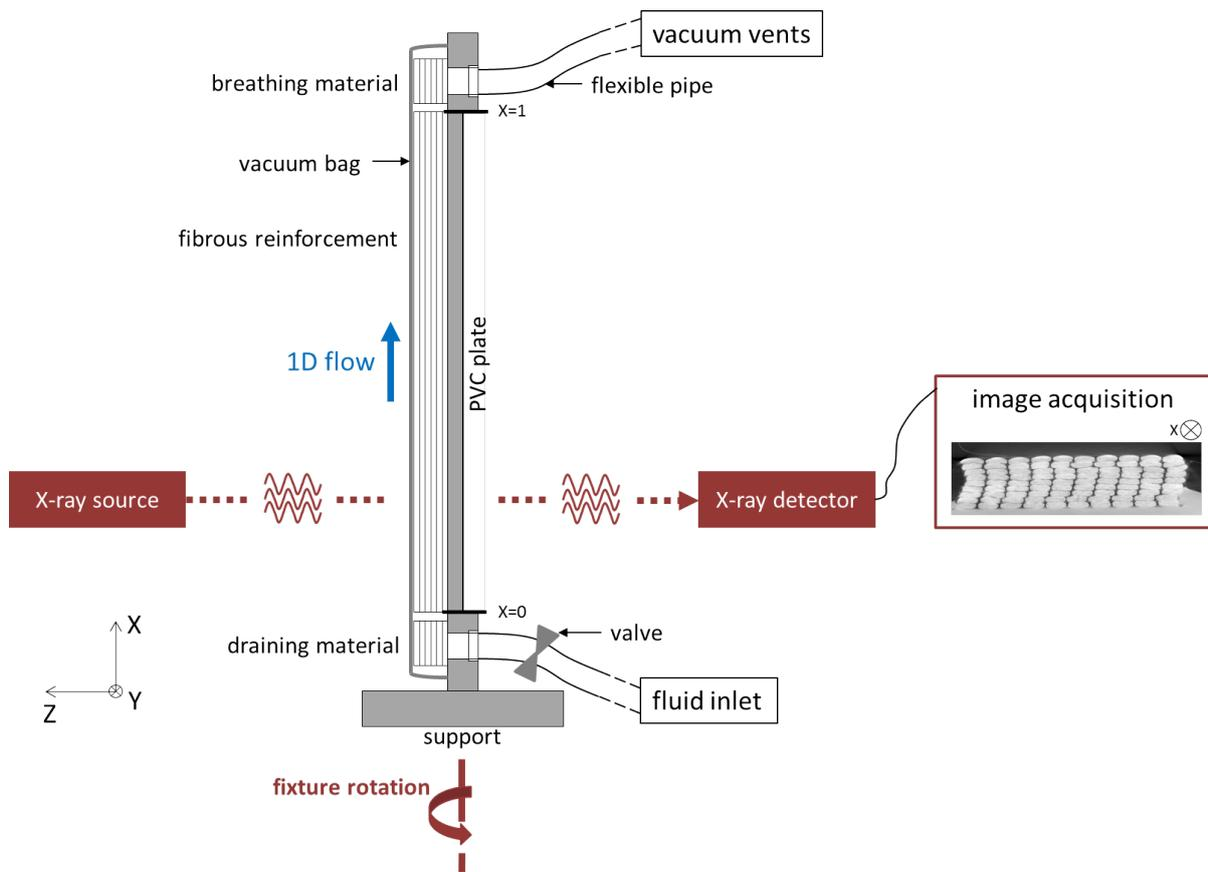
Figure I.15: Schematic view of the *Macro-meso-scale setup*: acquisition equipment effects (in red) and infusion setup (in grey)
