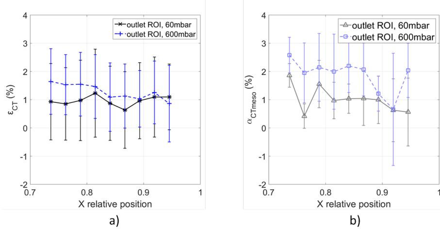
Figure I.50: Computation of the macroscopic decompaction (vertical vacuum bag displacement  $\bar{\epsilon}_{CT}$ , a) and the mesoscopic decompaction (tows area evolution  $\bar{\alpha}_{CTmeso}$ , b) for the outlet ROI, at 60 and 600 *mbar*.
