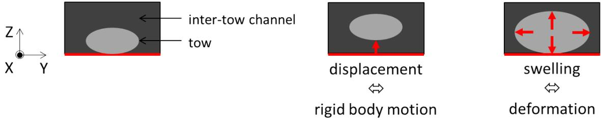
Figure I.1: Illustration of the impact of tow displacement and deformation on the microstructural reorganization
