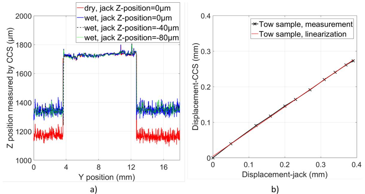
Figure III.16: Calibration at saturated state: a) detections of the bottom platen displacement when the fluid is in the pool. b) Correction curve of the overall system between the imposed displacement by the jack and the one measured by the CCS.
