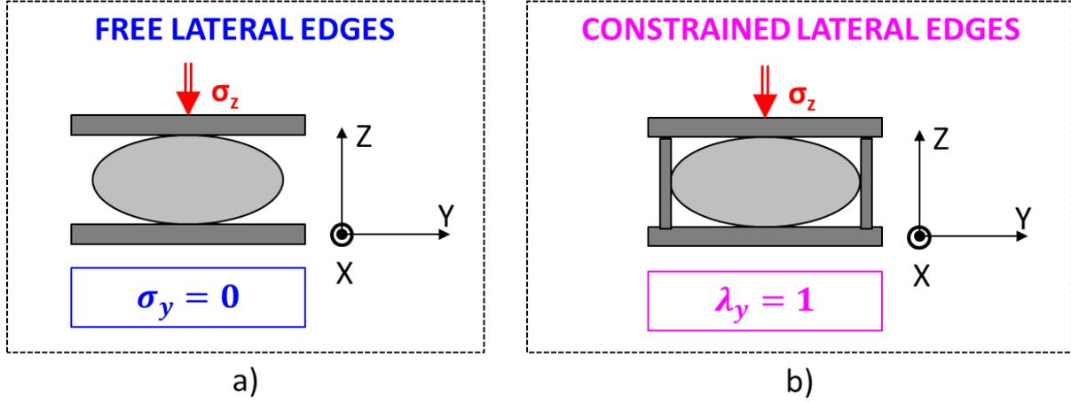
Figure III.27: Cross-section of a single tow subjected to a transverse compressive loading ( $\sigma_z$ ): a) free lateral edge boundary condition. b) constrained lateral edge boundary condition.
