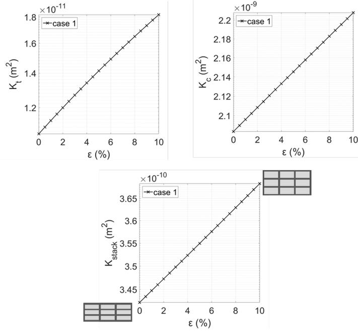
Figure II.11: Tows, inter-tow channels and stack permeability evolutions with the macroscopic decompaction  $\varepsilon$ , when the microstructural evolution follows the *Case 1*
