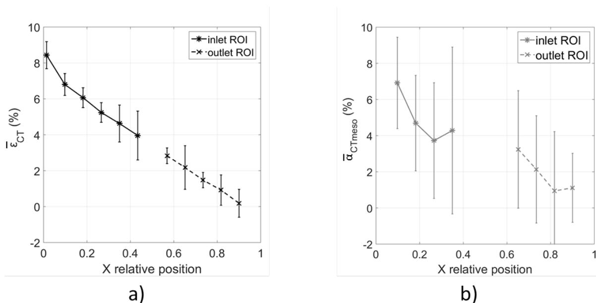
Figure I.38: Comparison between the macroscopic decompaction (vertical vacuum bag displacement) and the mesoscopic decompaction (tows area evolution): a) macroscopic decompaction. b) mesoscopic decompaction.
