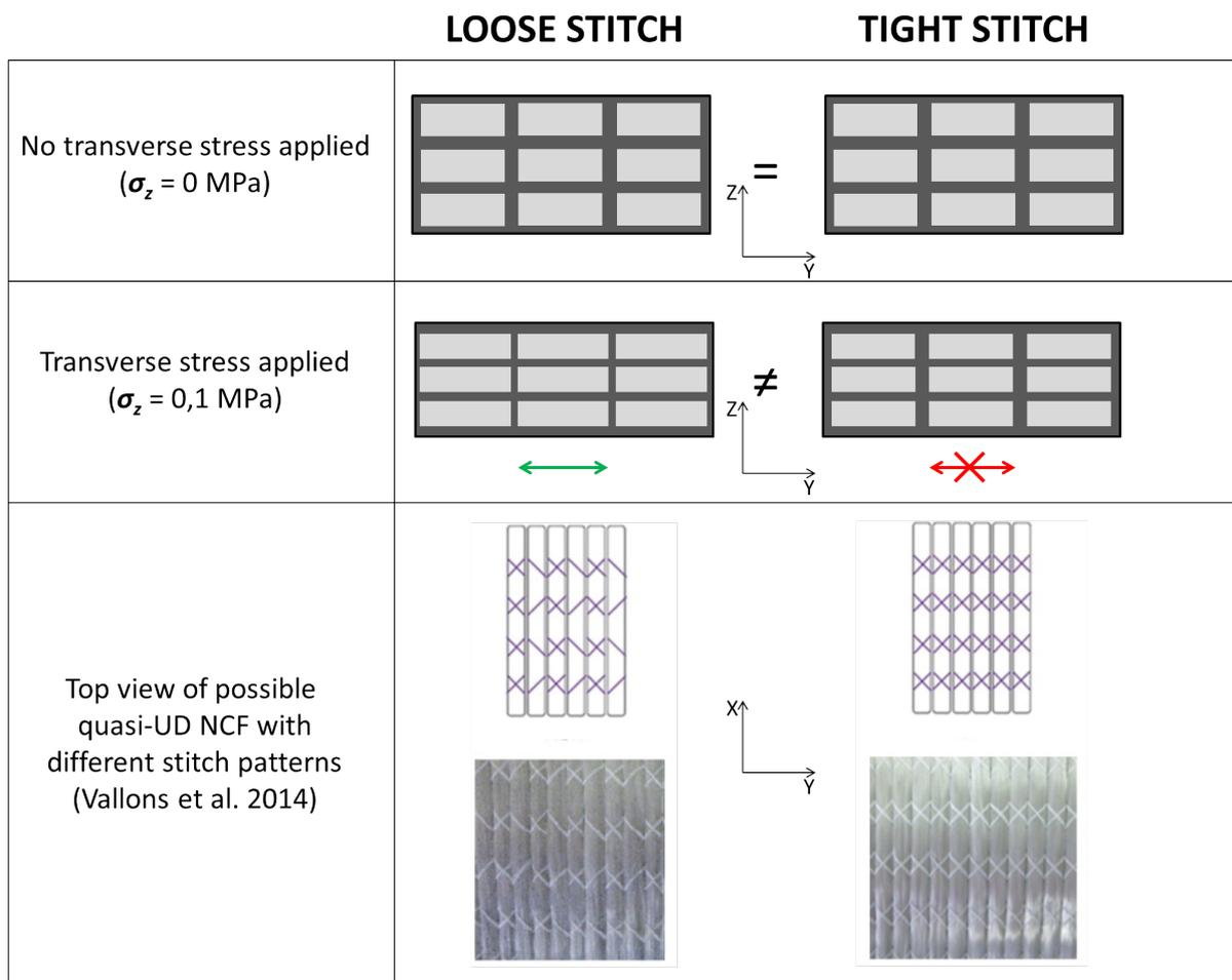
Figure III.21: Schematic view of the possible microstructural evolution during the loading phase of stacks of quasi-UD NCFs with a loose or a tight stitch
