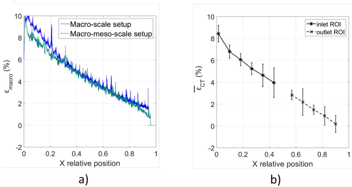
Figure I.28: Macroscopic decompaction gradient: a) using the *Macro-scale* methodology (confocal chromatic scanner). b) using the *Macro-meso-scale* methodology (CT-scan) and the *Macro-meso-scale* setup.
