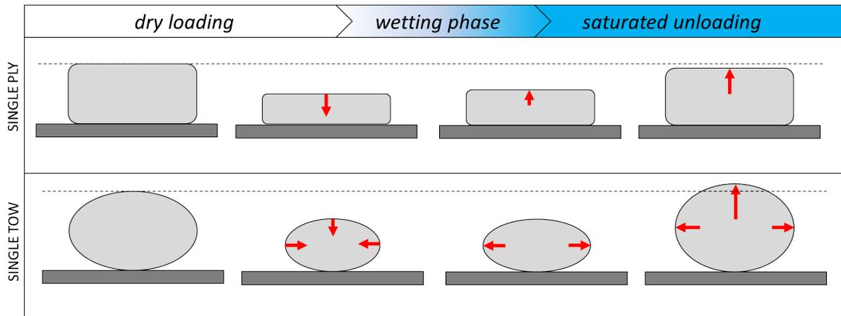
Figure III.13: Schematic view of the width and thickness evolutions of the two considered samples during the three main stages of the infusion process: a single ply of quasi-UD NCF and a tow extracted from this quasi-UD NCF
