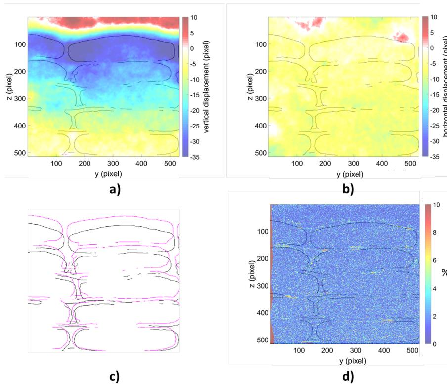
Figure I.47: Displacement fields between the dry and the saturated states at an X-position near the fluid inlet ( $X=0.04$ ): a) Vertical microstructure displacement (Z-axis) in voxel. b) Horizontal microstructure displacement (Y-axis) in voxel. c) Visualization of the microstructure evolution (in black: dry state, in pink: saturated state. d) Error of the Thirion algorithm for the considered images.
