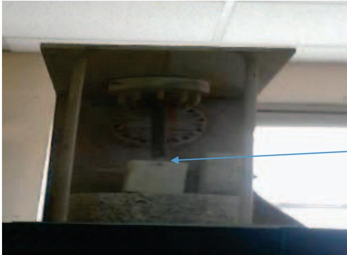
This part of the RMM was initially made from rock, but after testing in stage 4 of NDPM, it did not work as intended so the group repeated the NDPM cycle and used the 3D printer to print a replacement part made from PLA filament.
