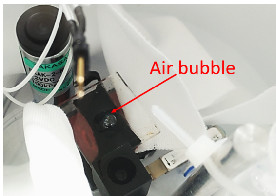
Figure 9.20: An image of the pico-flow cell while degassing by vacuum pump. The bubbles are visible coming out of the device.
