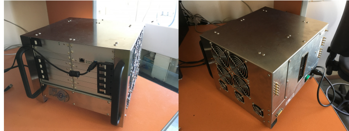
Figure 2.13: ULA-OP256 research scanner.
