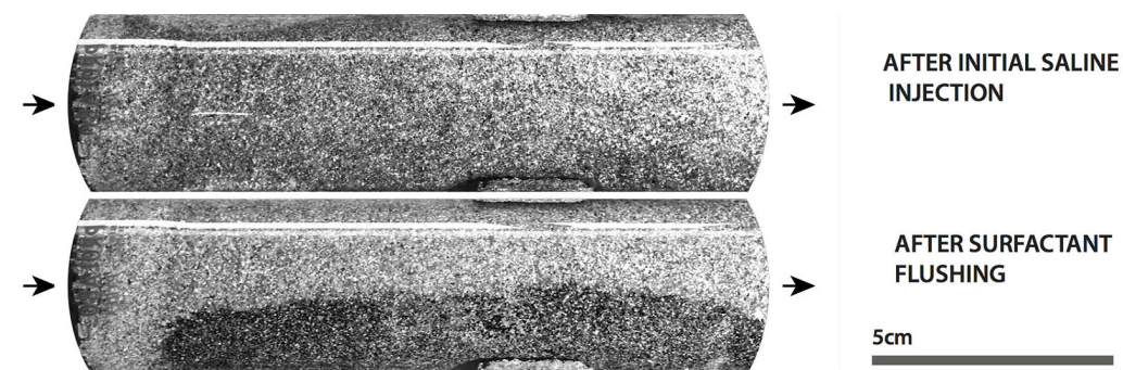
Figure 8.9: Initial (top) and final (bottom) DNAPL repartition for SF without foam.
