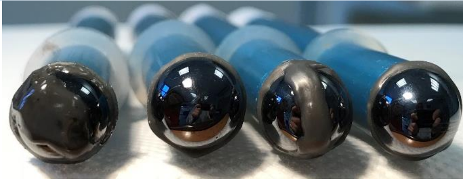
Figure IV.26. Photos showing the state of the synthesized membranes (45AgI-27.5HgS-18As 2 S 3 -9.5GeS 2 ) after calibration.
