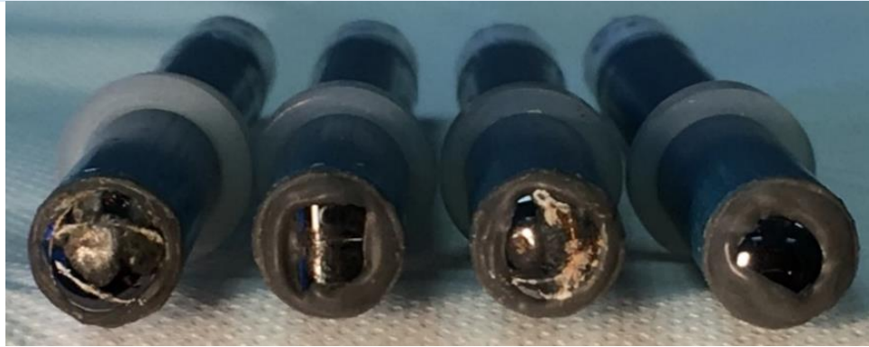
Figure IV.25. Photos showing the state of the synthesized membranes (30AgI-35HgS-35GeS 2 ) after calibration.
