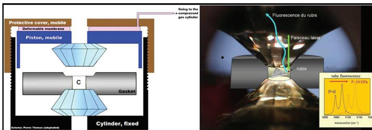
Figure 9 – Block diagram of the diamond anvil cell. This consists of three main parts: the piston and the cylinder which form the body of the cell, and the cover containing a metallic membrane.
