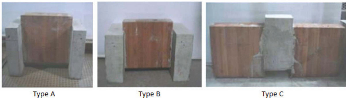
Figure I-16 : Configuration des éprouvettes Push-out [Carvalho and Carrasco, 2010]
