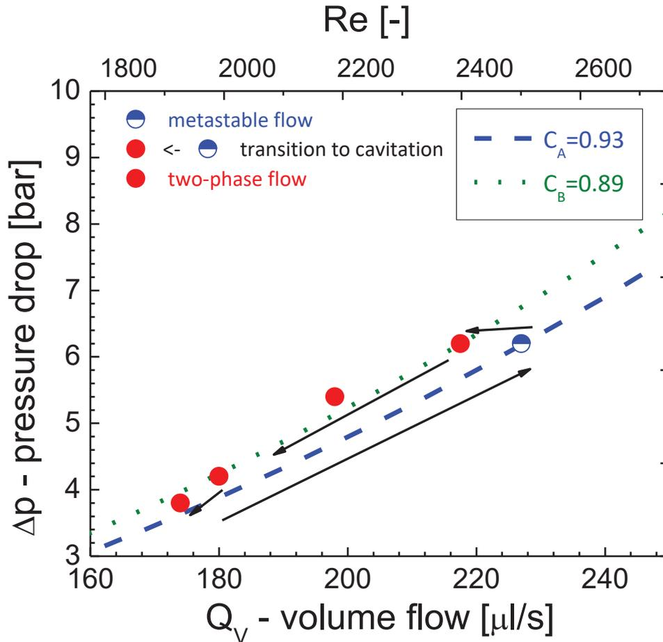
Figure 2.8 -  $\Delta p$  to  $Q$  and  $Re$  graph, showing the hysteresis and metastability in microfluidic channels when using clean, well filtered liquid.  $Re$  is the Reynolds number (see page 24). Adapted from [85].
