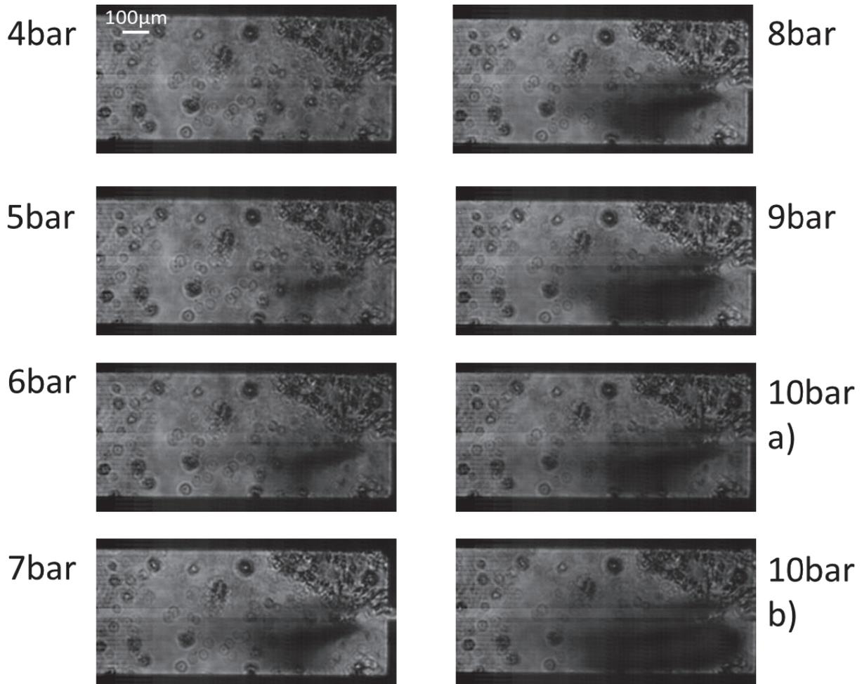
*Figure 2.17 - Images averaged over 1000 frames at 150kHz. At 10 bar the two regimes are shown; a) the typical flow and b) the bubble coalescence.*
