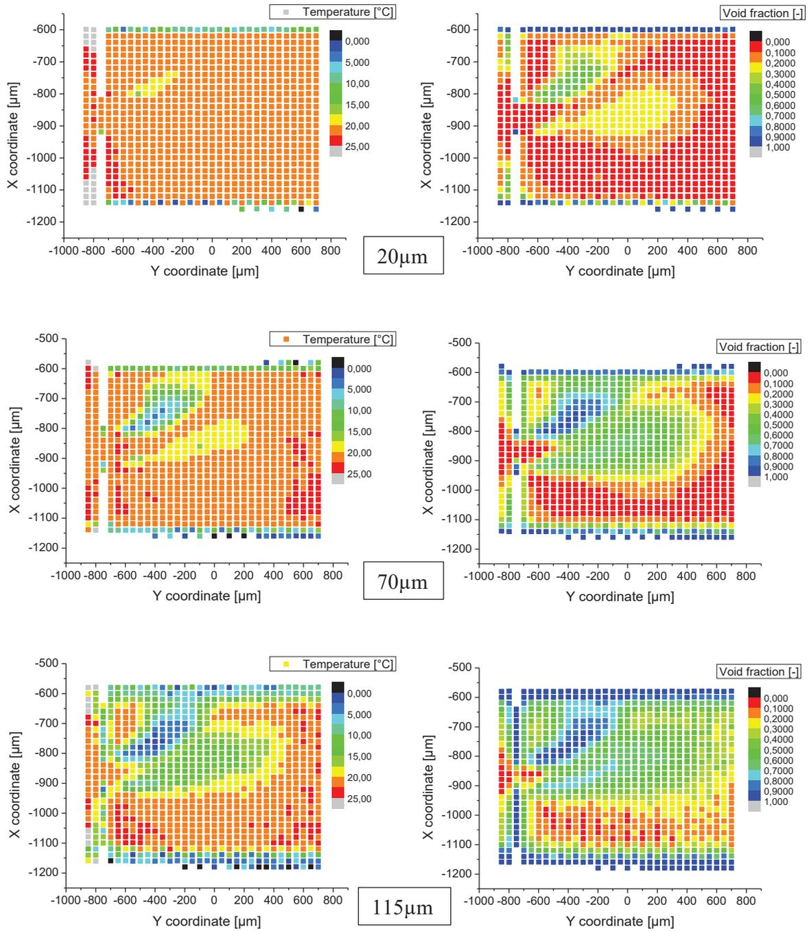
Figure 4.4 - MD L4 at 10bar; temperature (left) and void fraction (right) mapping at 20, 70 and 115μm from glass (order from top to bottom). Flow is from left to right at 10 bar driving pressure. Diaphragm walls are best seen on lower right temperature map.
