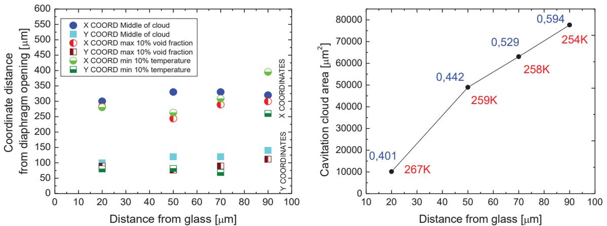
Figure 4.12 - figure on left showing the coordinates of the area analysis from diaphragm opening along the height of the MD L6 channel at 10 bar driving pressure. Figure on right showing the cavitation cloud, its average void fraction (blue value) and the temperature drop (red value).
