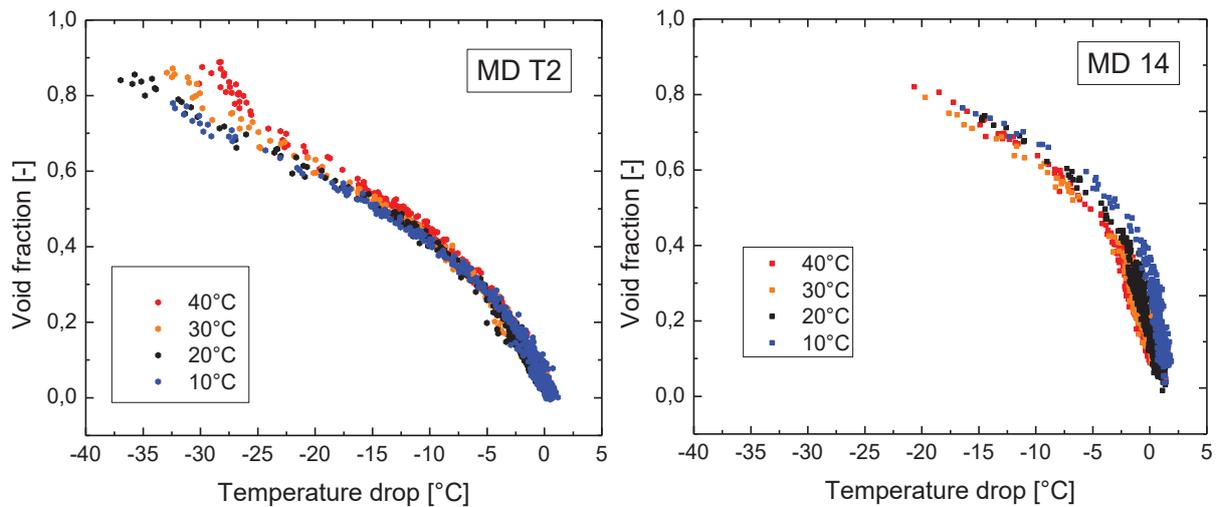
Figure 4.20 - Scatter plot for MD T2 and 14 at 8bar and the mid-height of the channel with varying inlet liquid temperature.
