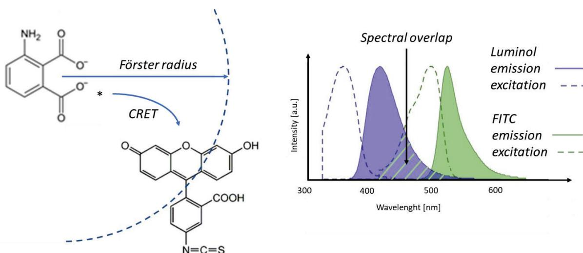
Figure 7.4 - CRET mechanism for luminol/FITC pair. On left the Forsters distance requirement and on the right the spectral overlap requirement.
