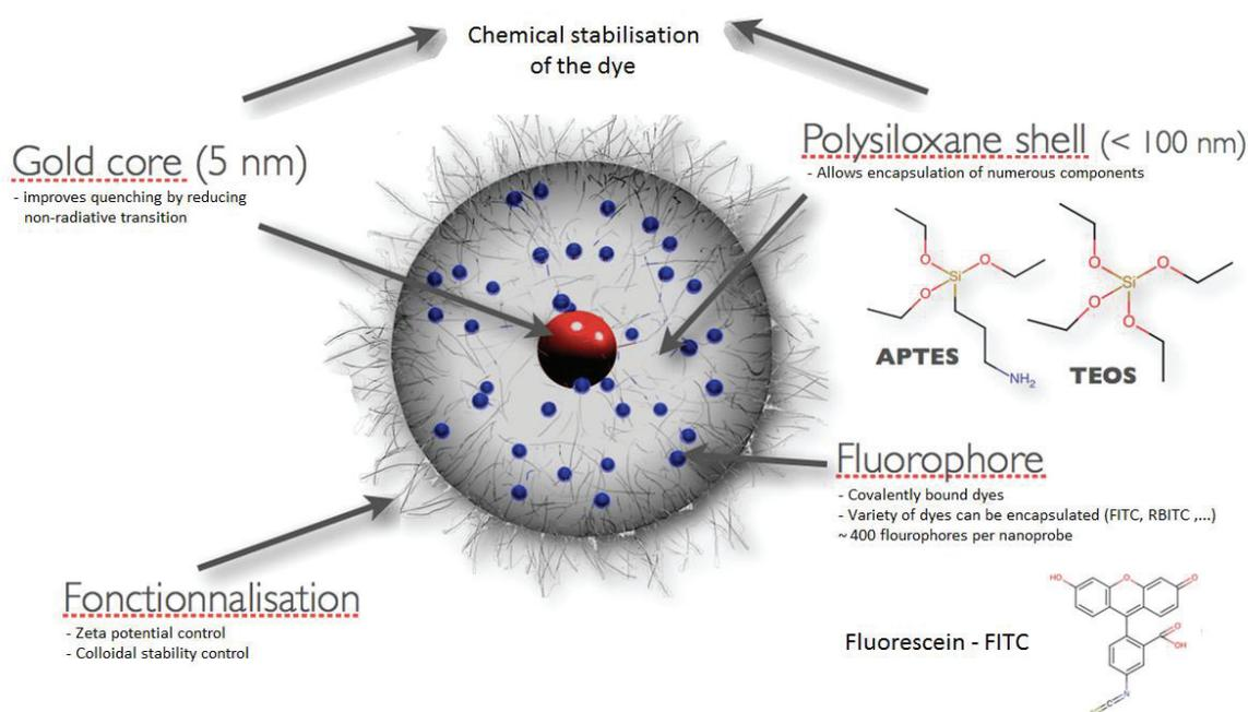
Figure 3.23 - temperature sensitive fluorescent (Au:SiO<sub>x</sub>) nanoparticles; 5nm gold core with a ~25-30nm thick poly silica shell containing fluorescent dyes (FITC), with functionalization on the surface to prevent precipitation. Internal laboratory data.
