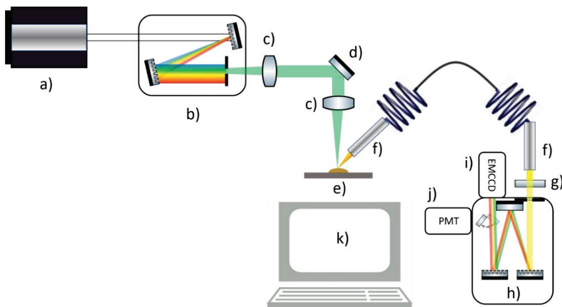
*Figure 3.8 - Excitation emission spectrometer. a) to d) – laser driven xenon lamp with monochromator for excitation wavelength selection; e) sample; f) to j) – acquisition line (optical fibre, analysis monochromator, detection device (EMCCD and PMT)); k) excitation/emission spectrometer control. Devices specified in Table 7.*
