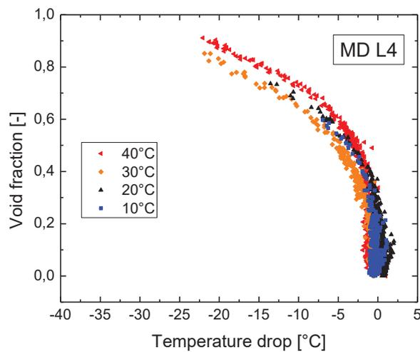
Figure 4.21 - Scatter plot for MD L4 at 8bar and the mid-height of the channel with varying inlet liquid temperature.
