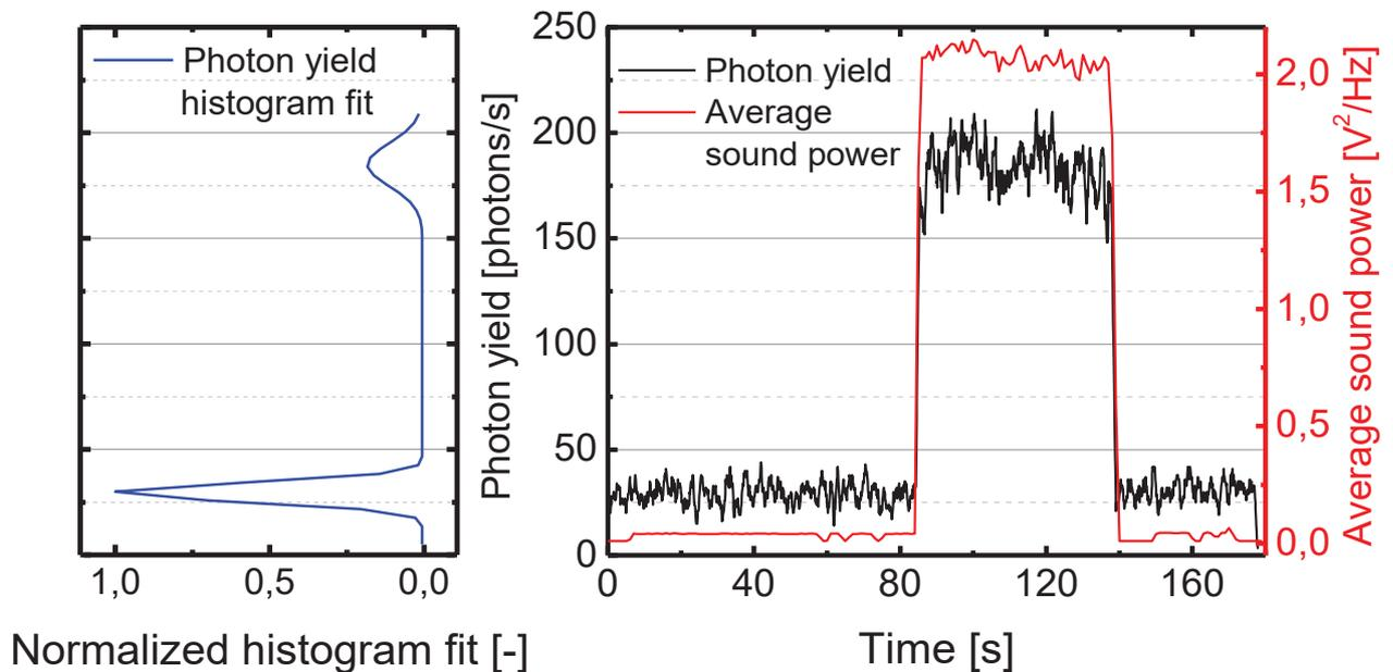
*Figure 5.5 - MD L3 at 10bar driving pressure. The graph presents a typical measurement series, producing a histogram (blue line) of the CL signal (black line) on the right. The red signal presents the sound power curve, corresponding nicely to the CL signal.*
