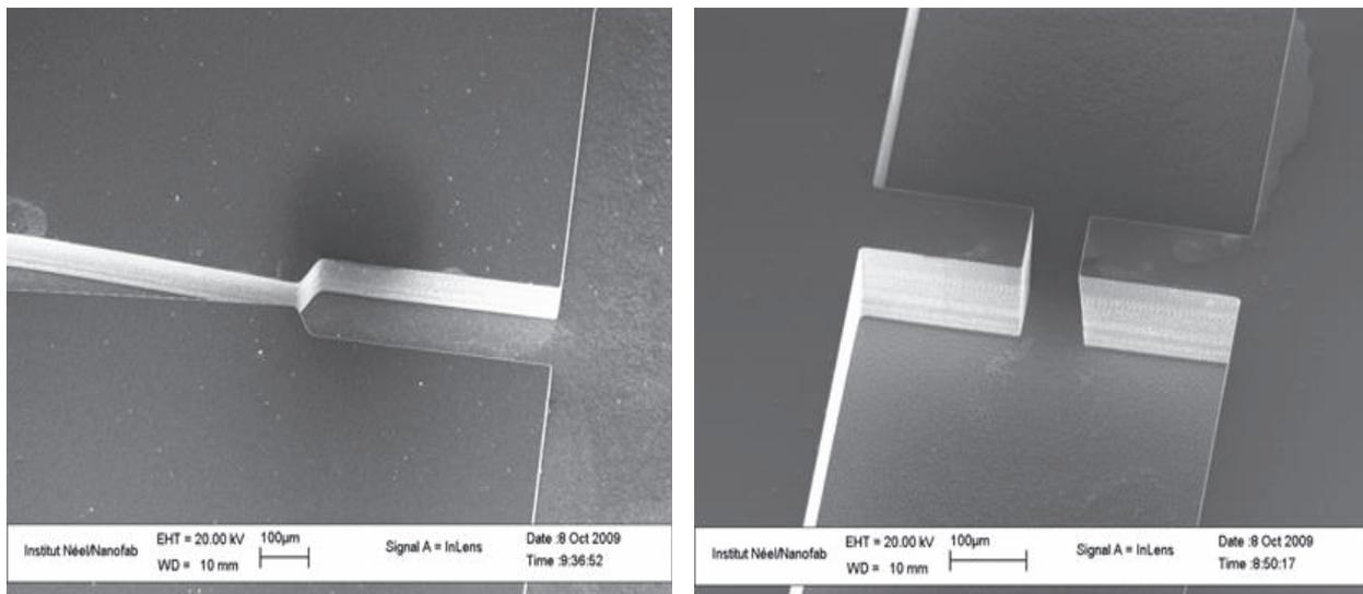
*Figure 2.10 - Scanning electron microscope images of channels after etching (step 2). The high aspect ratio and nearly perpendicular walls can be observed [84].*
