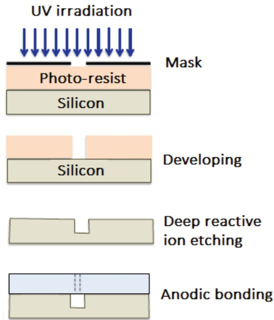
Figure 2.9 - Microchannel manufacturing phases. Adapted from [86].
