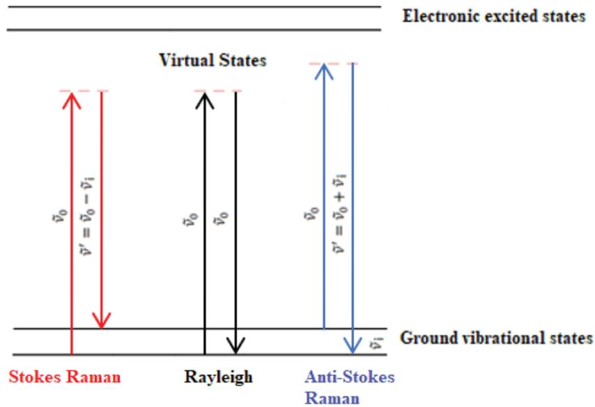
Figure 4.25 - Rayleigh scattering (elastic), Stokes (red shift) and Anti-Stokes (blue shift). From the intensity of the Anti-Stokes and Stokes peaks, one can probe the ground vibrational state population, which would depend of the Boltzmann distribution (temperature dependent).
