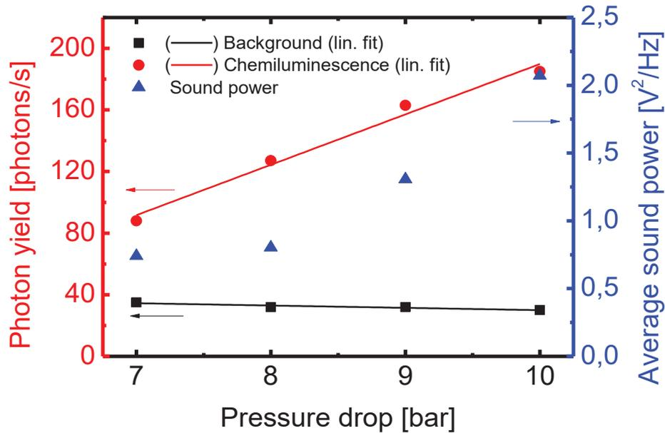
Figure 5.9- MD L3 CL yield and noise sound power as a function of the driving drop.
