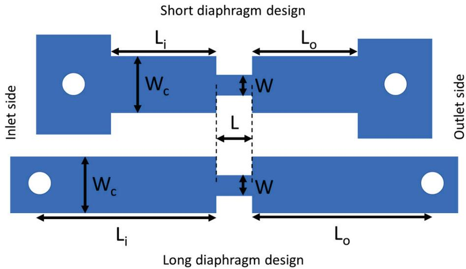
Figure 2.12 - Short and long microdiaphragm design schematic. The geometric parameters  $W_c$  is fixed for all channels at  $500\mu\text{m}$  ( $\pm 10\mu\text{m}$  between channels). For long diaphragm  $L_i=15000\mu\text{m}$  and  $L_o= 25000\mu\text{m}$ , while for the short diaphragm they are equal at  $1500\mu\text{m}$ . Other variable parameters are shown in Table 1.
