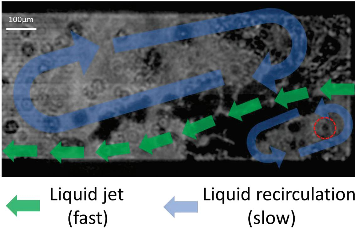
*Figure 2.18 - The two main recirculation zones in typical cavitating flow of a microdiaphragm (6bar driving pressure). The red dashed circle indicating the residual gas bubbled, most likely produced by degassing in the cavitating flow. These bubbles recirculate and get injected in the shearing flow, serving as nuclei and sustaining the cavitating flow.*
