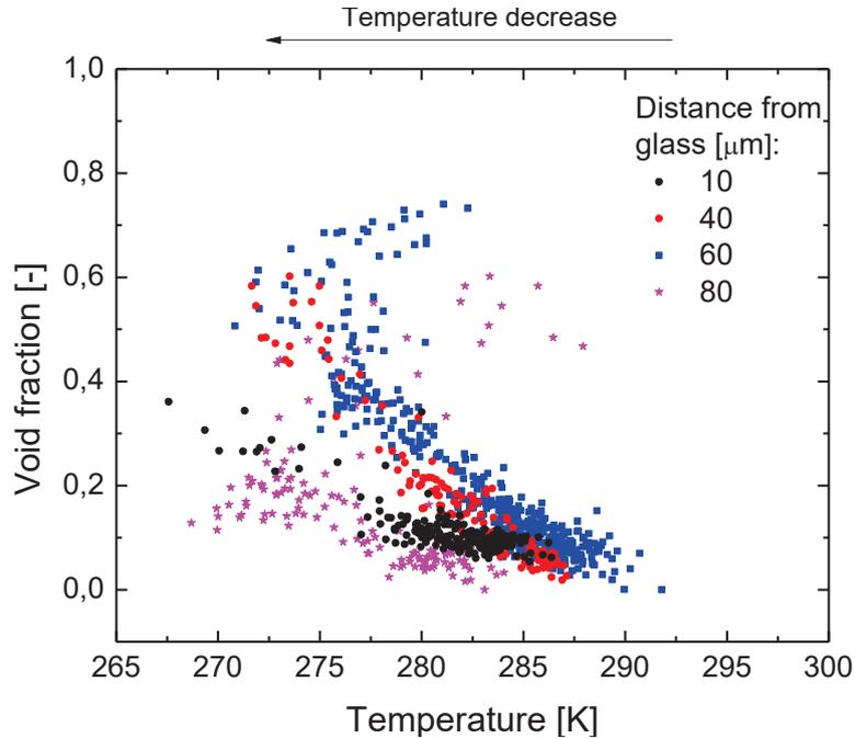
Figure 4.7 – MD10 temperature vs void fraction plot, 10bar driving pressure measured at different heights in the channel. The legend indicates the  $z$  plane height in reference to the glass liquid interphase, expressed in micrometres.
