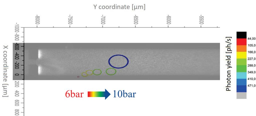
*Figure 5.15 - 2D Gaussian fit of CL mapping data of the L4 channel. The maximum coordinates and intensity indicated by the circles are overlapped on channel long exposure time image. The circle size and colour indicate the photon yield; The low intensity red circle at 6bar progressively increasing with driving pressure to the high yield blue circle at 10 bar.*
