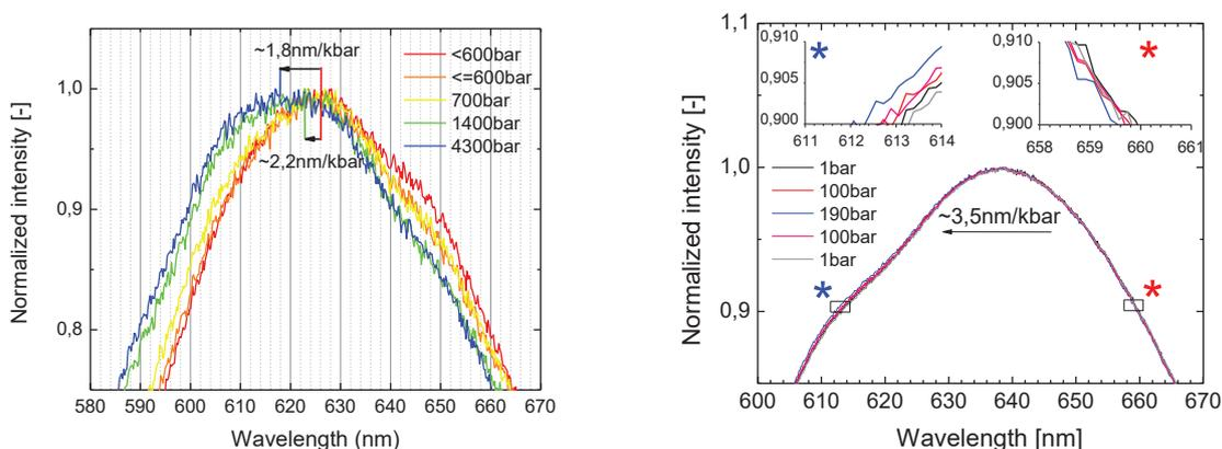
Figure 3.22 - Luminescent response at increased pressure for  $[Au(I)(p-SPhCOOCH_3)]_n$ . On left the diamond anvil cell results with pressures up to 4300bar in squalene medium. On right the exposure to 200bar of pressure in nitrogen gas medium.
