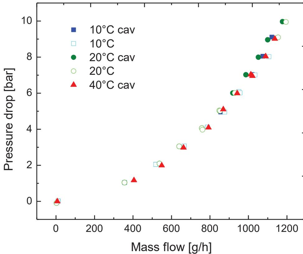
Figure 2.14 - Pressure vs mass flow curve diagram ( $p-Q_m$ ) for the T2 short diaphragm microchannel with varying temperature. Coloured symbols show two-phase flow while hollow ones show single phase flow.
