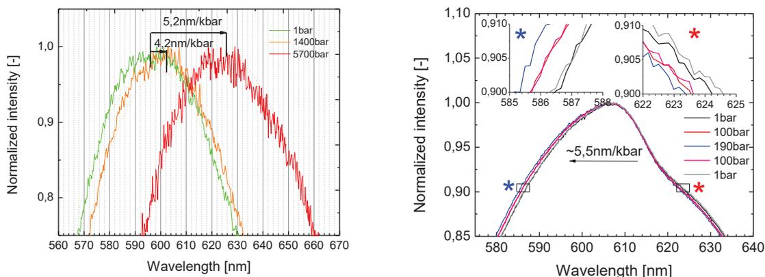
Figure 3.21 - Luminescent response at increased pressure for  $[Au(I)(p-SPhCOOH)]_n$ . On left the diamond anvil cell results with pressures up to 5700bar in squalene medium. On right the exposure to 200bar of pressure in nitrogen gas medium.
