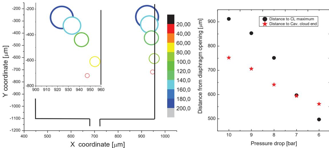
*Figure 5.18 – MD 14 coordinates of 2d gaussian peak fit to CL mapping data on left. On right plotted distance from the diaphragm opening. Distance to CL 2d gaussian fit peak (data on left) compared to the distance to the end point of the cavitation cloud (void fraction mapping - 4.2.4).*
