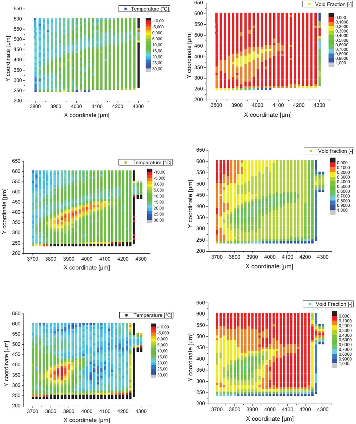
Figure S.3 - text MD 10 at 8 bar driving pressure. Analysis at different height; 20, 50 and 80 from glass (in descending order). Left plots are temperature and right are the void fraction maps. Flow is from right to left.
