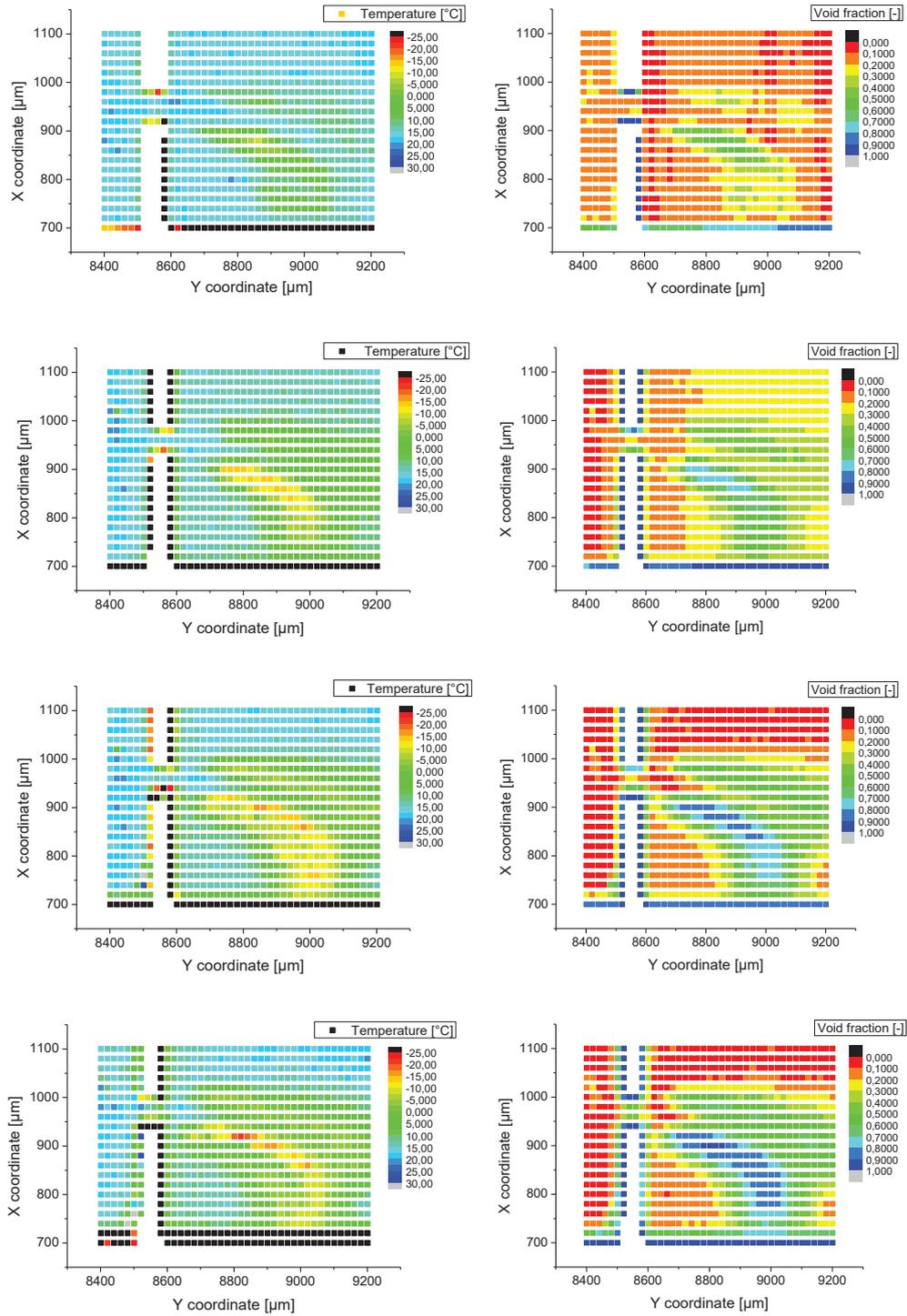
*Figure S.2 - MD L6 temperature (left) and void fraction (right) mapping at 20, 50, 70 and 90 μm from glass (order from top to bottom). Flow is from left to right at 10 bar driving pressure.*
