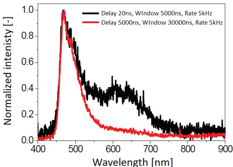
Figure 3.19 - Timer resolved spectroscopy data of  $[\text{Au(I)}(\text{p-SPhCOOH})]_n$ ; in the legend the nanosecond time for the delay from pulse, the temporal window of the observation and the laser pulse rate is shown. Adapted from [131].
