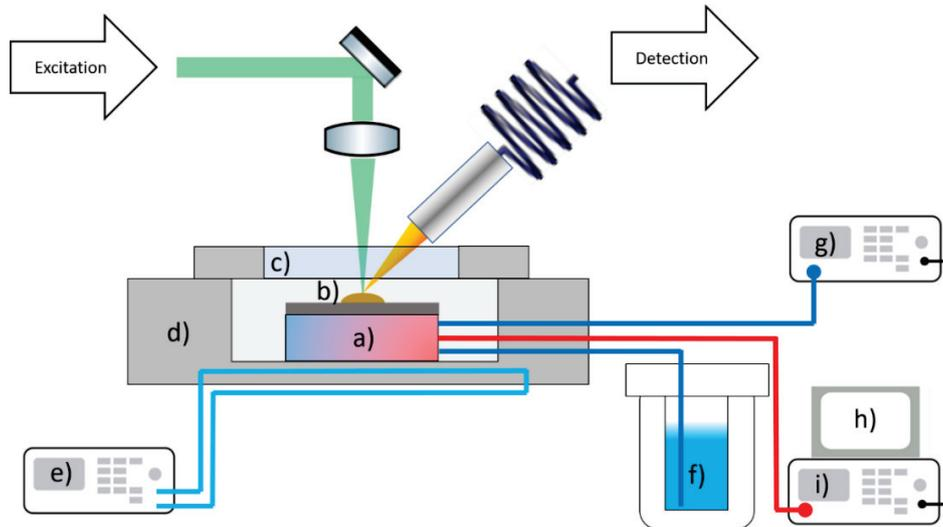
Figure 3.12 – Linkam temperature control system (heating/cooling stage); a) Linkam THMS-600 heating/cooling sample holder with liquid nitrogen lines and electrical resistive heater, b) sample on silicon wafer, c) cover with sapphire optical window, d) temperature control stage housing with water recirculation, e) water recirculation system, f) liquid nitrogen Dewar; Linkam T95-PE system: g) liquid nitrogen pump, h) control module and i) temperature control system.
