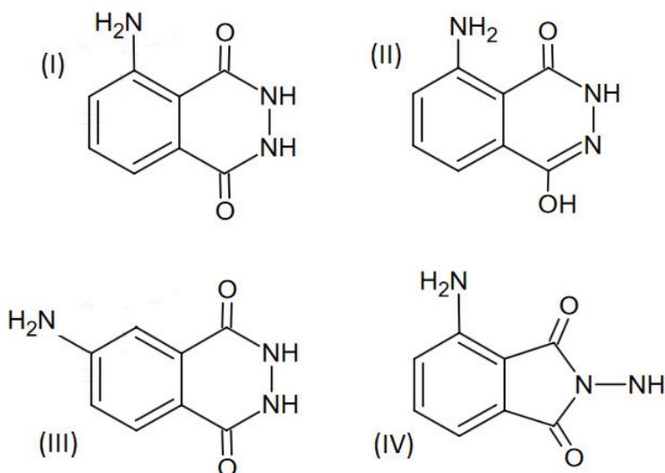
Figure 5.2 - luminol isomers and tautomer (combined from [171], [175]).
