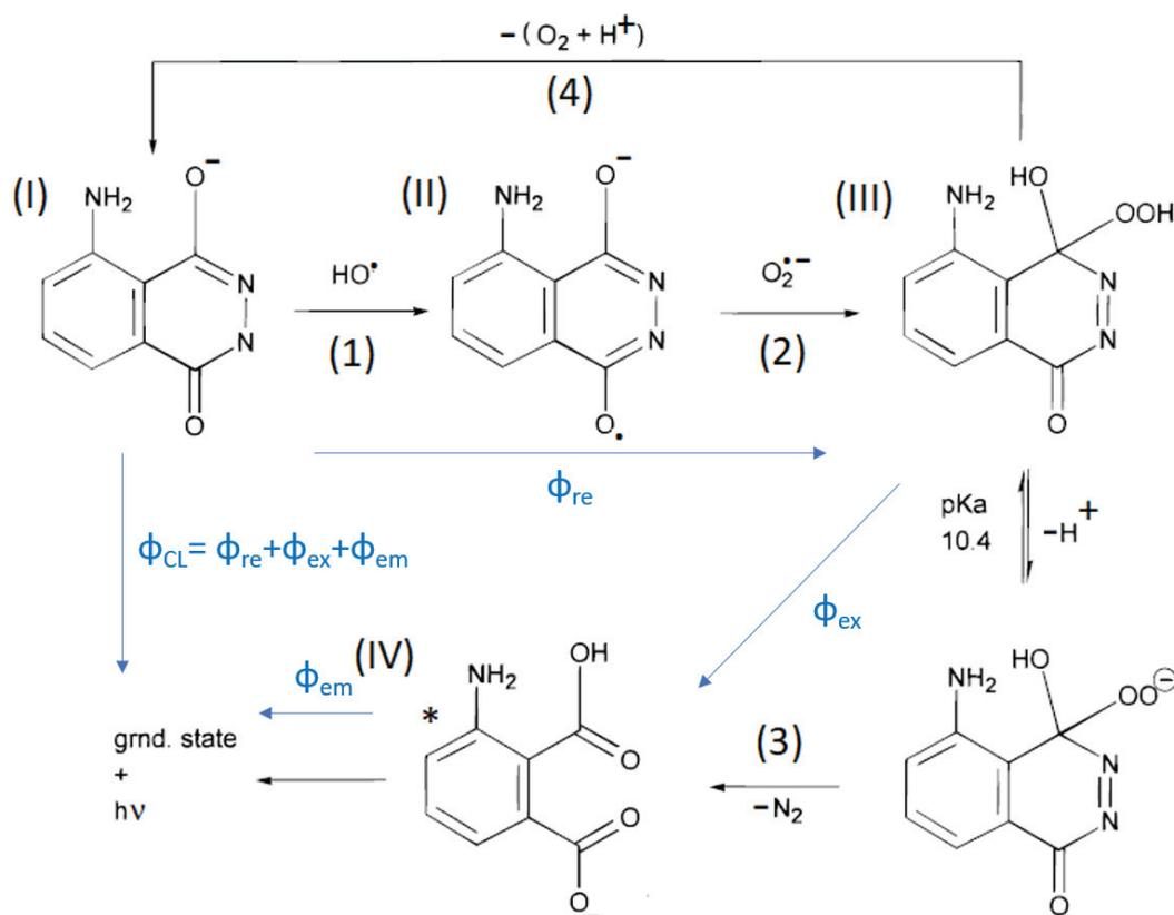
Figure 5.3 - LCL pathway for luminol oxidation by hydroxyl radical and super-oxide ion from a cavitation bubble (adapted from [162]).
