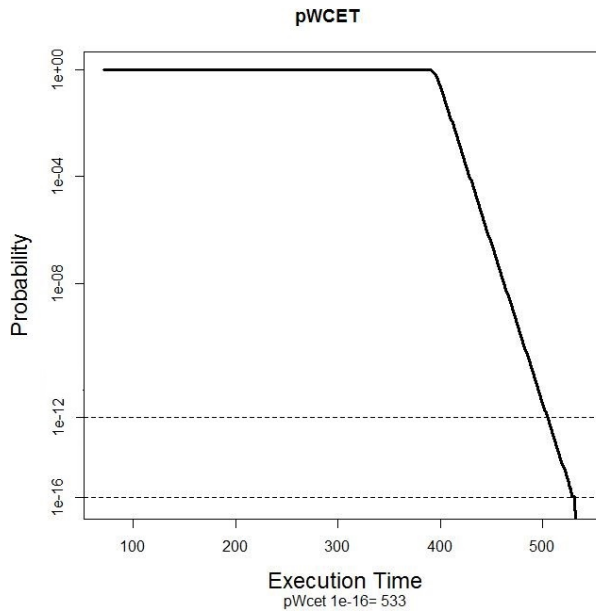
Figure 5.7: pWCET estimation from dependent execution times of the program prime on the Aurix architecture.
