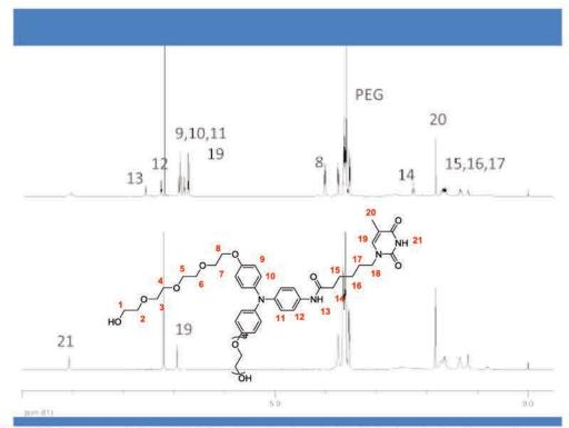
Figure S3| NMR spectra of 4PEGTAMT before (top) and after light irradiation (bottom).
