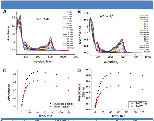
**Figure 64**| A. UV-vis-NIR spectra of **TAMT** for increasing irradiation times. B. UV-vis-NIR spectra of **TAMT-Hg(II)** complex for increasing irradiation times. C-D. Evolution of the absorbance at C. 782 nm for **TAMT-Hg(II)** complex (black) and 805 nm for **TAMT** (red) and D. at 382 nm for **TAMT-Hg(II)** complex (black) and **TAMT** (red) as a function of irradiation time (c = 0.1 mM in chloroform).
