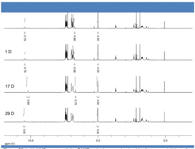
Figure S7 | 1H NMR spectrs of the TAMT-melamine complex in chloroform recorded just after dissolution; after 1 day and after 17 and 29 days.
