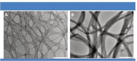
**Figure 76**| TEM images of **TAMG** from a toluene solution in the absence of KPF $_6$  (A) and in the presence of KPF $_6$  (B). (Scale bar:  $1\mu m$ )
