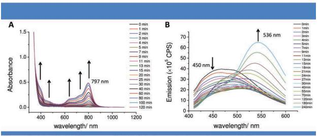
**Figure S4** | A. UV-vis-NIR spectra of **TAMaC** for increasing irradiation times. B. Fluorescence spectra of **TAMaC** for increasing irradiation times ( $\lambda_{exc.} = 400 \text{ nm}$ ) (c = 0.1 mM in chloroform).
