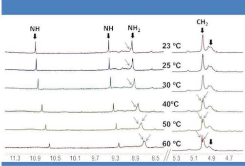
Figure 70| Variable-temperature NMR spectra of a 4 mM solution of TAMG-KPF6 in THF.
