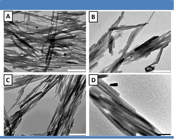
**Figure 61**| TEM images of the **TAMT**-melamine complex in toluene at concentrations lower than the gelation concentration: 20 mM (A,B), 10 mM (C,D). (Scale bar: A-C:  $1\mu m$ ; D: 200 nm)
