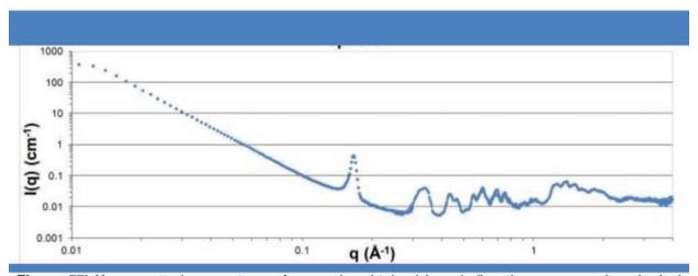
Figure 57| X-ray scattering spectrum of a powder obtained by grinding the macroscopic spherical aggregates.
