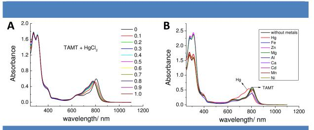
**Figure 66**| A. UV-vis-NIR absorbance spectra of a light-irradiated solution of **TAMT** upon the addition of mercury (0-1 eq.). B. UV-vis-NIR absorbance spectra of pure **TAMT** and **TAMT** mixed with different metals (0.5 equivalent) (c = 0.1 mM in chloroform).
