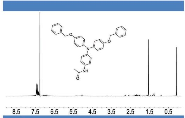
Figure S9 | <sup>1</sup>H NMR spectrum of BATA after the addition of HgCl<sub>2</sub> in chloroform.
