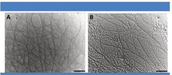
**Figure 75**| TEM images of **TAMG** from a THF solution in the absence of KPF<sub>6</sub> (A) and in the presence of KPF<sub>6</sub> (B). (Scale bar:  $1\mu m$ )
