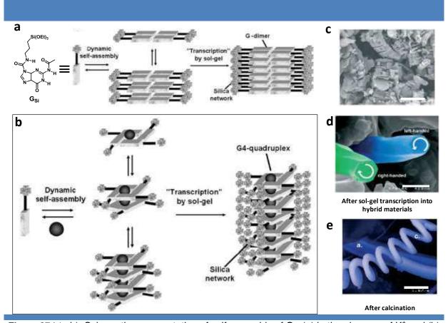
**Figure 27** | (a-b). Schematic representation of self-assembly of  $G_{Si}$  (a) in the absence of  $K^+$  and (b) in the presence of  $K^+$ . (c-e). SEM images of (c) the G-dimer hybrid in the absence of  $K^+$  after calcination (scale bar: 2  $\mu$ m); (d) G-quadruplex hexagonal nanorods resulting from sol-gel transcription in the presence of  $K^+$  (scale bar: 429 nm); (e) silica nanofibers and microsprings after calcination (scale bar: 1.67  $\mu$ m). Adapted from reference 145.
