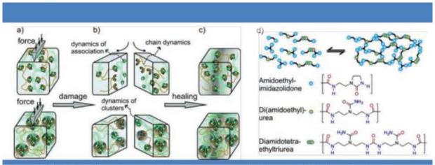
**Figure 9** | (a)-(c) Self-healing mechanism for a supramolecular material; (d) synthesis pathway and molecular structure of self-healing rubber. Reproduced from references 46,47.
