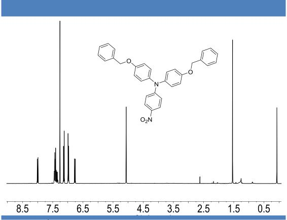
Figure S8 | <sup>1</sup>H NMR spectrum of compound 10 after the addition of HgCl<sub>2</sub> in chloroform.
