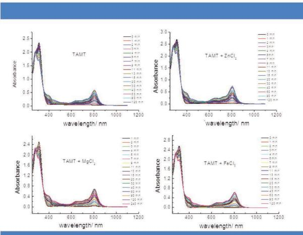
Figure S10 | UV-vis-NIR spectra of TAMT upon light irradiation in the absence or in the presence of different metal ions.
