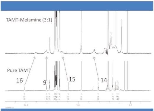
Figure 59| NMR spectra of the TAMT-melamine complex and pure TAMT in d<sub>8</sub>-toluene at 20mM.
