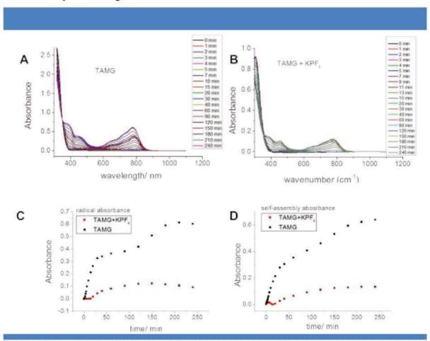
**Figure 74**| A-B . UV-vis-NIR spectra of **TAMG** in the absence (A) or in the presence of potassium salt (B) for increasing irradiation times. C-D. Evolution of the radical absorbance (C) and the self-assembly absorbance (D) for **TAMG** and **TAMG**-KPF $_6$  as a function of irradiation time (c = 0.1 mM in chloroform).
