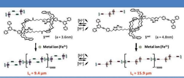
**Figure 5** | Schematic representation and chemical structures of a terpyridine-terminated supramolecular polymer made of contractile [c2]daisy chains units. Their collective contraction/extension changes the average size of the polymer chain.
