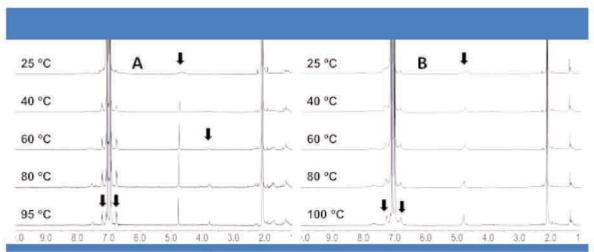
**Figure S12** | Variable-temperature <sup>1</sup>H NMR spectra of **TAMG** in the absence (A) and in the presence (B) of KPF<sub>6</sub> (4 mM solution in toluene).
