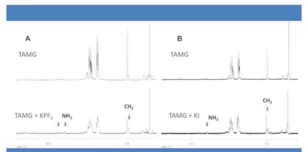
**Figure 69**| <sup>1</sup>H NMR spectra of **TAMG** and **TAMG**-KPF<sub>6</sub> complex (A, c = 4 mM in THF); **TAMG**-KI complex (B, c = 2.8 mM in THF) at room temperature.
