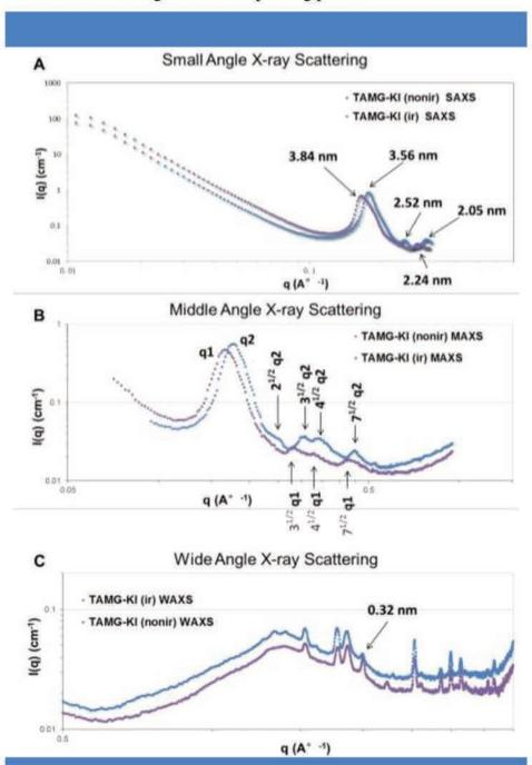
Figure 72| Powder SAXS (A) / MAXS (B) / WAXS (C) spectra of the **TAMG**-KI complex before (blue) and after (purple) irradiaiton with white light.
