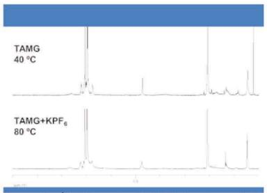
**Figure 68**| Variable-temperature <sup>1</sup>H NMR spectra of **TAMG** in the absence (top) and in the presence (bottom) of KPF<sub>6</sub> (4 mM solution in toluene).
