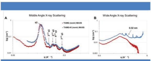
Figure 71| Powder MAXS (A) and WAXS (B) spectra of TAMG in the presence (blue) and in the absence (red) of KI.
