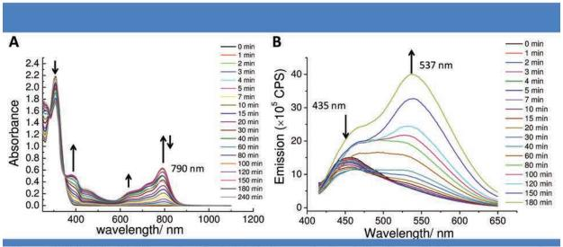
**Figure S5** | A. UV-vis-NIR spectra of **TAUPy** for increasing irradiation times. B. Fluorescence spectra of **TAUPy** for increasing irradiation times ( $\lambda_{exc.} = 400 \text{ nm}$ ) (c = 0.1 mM in chloroform).
