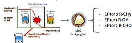
The formulation was heated to 90 °C followed by cooling to 60 °C. 3 times. During the 3rd cooling step, at 82 °C the active EP1010 was added, in the next cycle, EP1011 was added at 76 °C, following by EP1012 added at 75 °C. The system was diluted with 12,5 mL cold water (4 °C) in the last cycle at 55 °C leading to the formation of stable LNCs.
