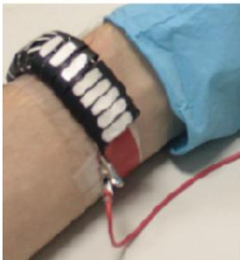
Figure 17: One possible configuration of the thermoelectric generator composed of the p- and n- legs from P3HT / carbon nanotubes nanocomposites. Each leg has a 5mm width and they are arranged in a wristband in order to harvest the thermal energy of the human body. 53
