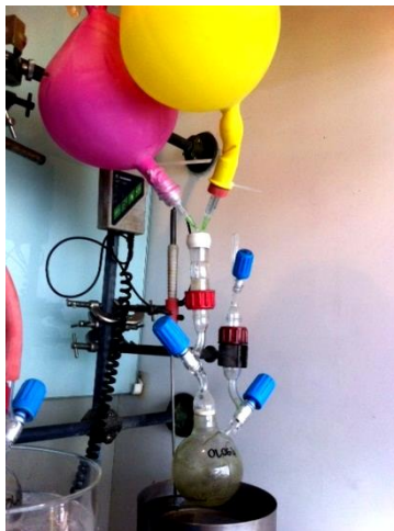
Figure ESI 6 - Round bottom flask containing a fritted glass filter to recycle the supported-TEMPO, with a system to attach the balloons containing oxygen or air.
