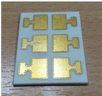
Figure 17: Substrat alumine Curamik
