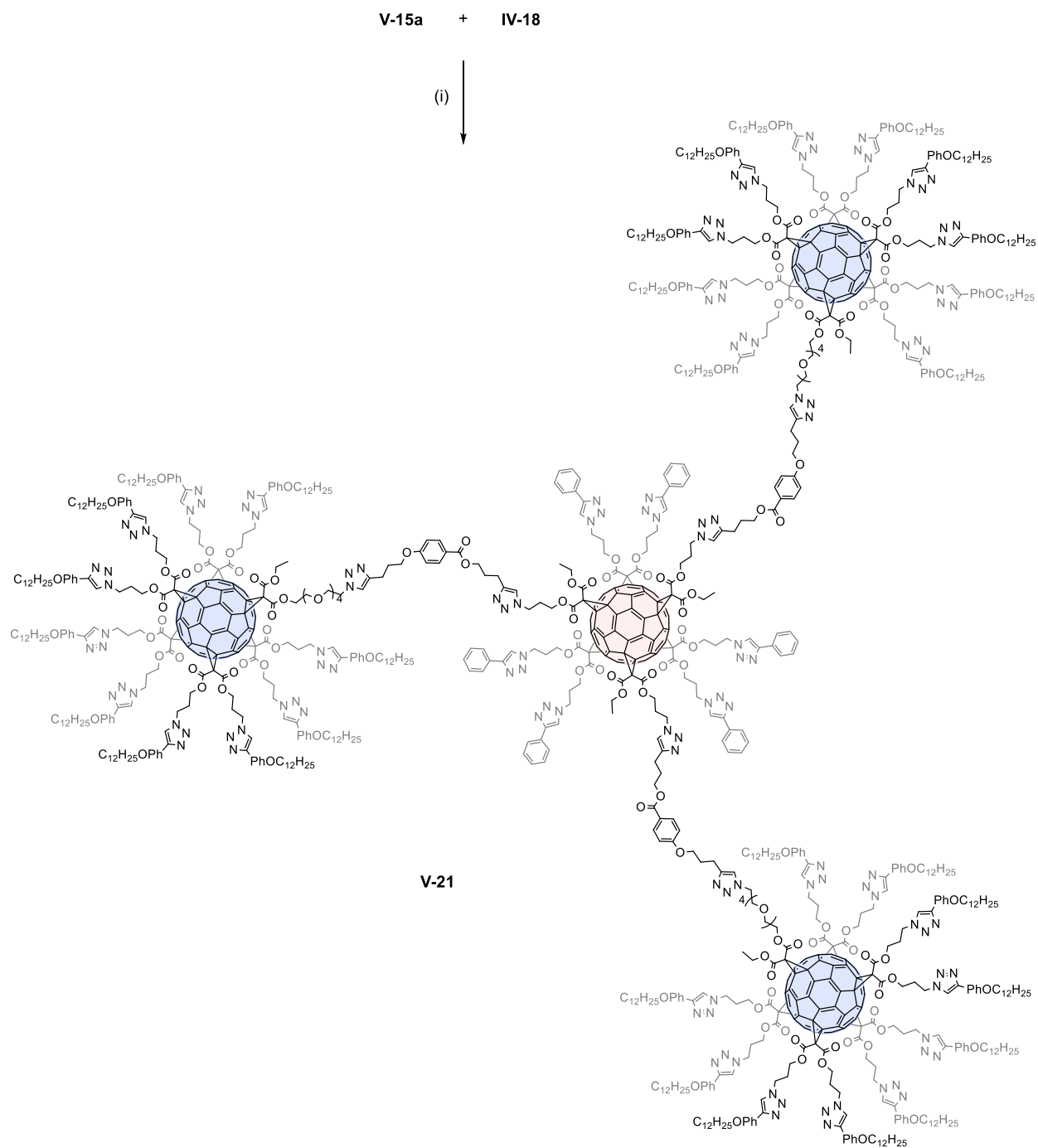
Scheme V-6. Reagents and conditions: (i) CuSO 4 ·5H 2 O, sodium ascorbate, CH 2 Cl 2 /H 2 O, 30 °C, 12 h (62%).
