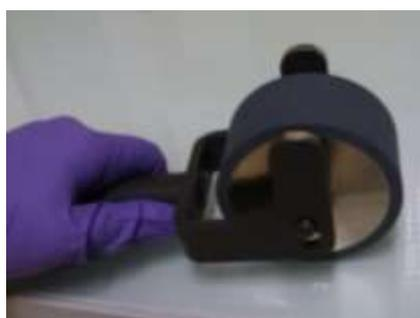
**Figure 2.5 The weighted hand roller used for laminating samples is shown. The gray, soft rubber coating on the metallic, heavy, steel roller is clearly visible in the image.**
