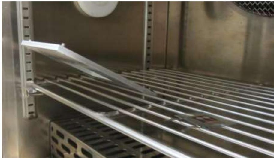
Figure 2.6 A sample for an optical calcium test (left) and an encapsulated OPV cell (right) are shown inside a humidity chamber.
