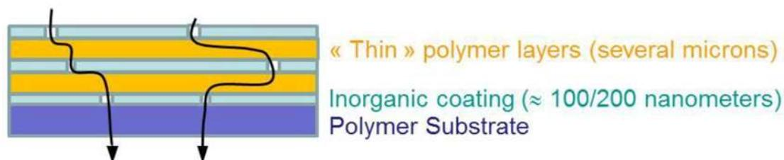
**Figure 1.11** The black arrows represent possible permeation pathways through a three dyad multi-layer barrier film. These pathways are tortuous as the permeating molecules cannot traverse the laminate in a straight line. Instead, the gas must permeate through each intermediate polymer layer along the impermeable inorganic barrier layers until it reaches another defect. This greatly increases the path length for permeation and therefore results in a low permeation rate.<sup>92</sup>
