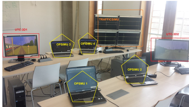
Figure 6.3 – ERTMS/ETCS Operational Simulator set-up: a picture, and its architecture listing the functions and different machines
