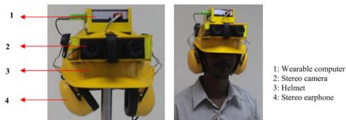
Figure 2.13 SVETA experimental system [42]
