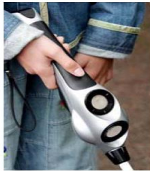
Figure 2.7 The UltraCane, University Leeds [36]
