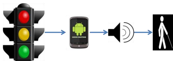
Figure 3.10 SEE-Phone in detecting traffic light
