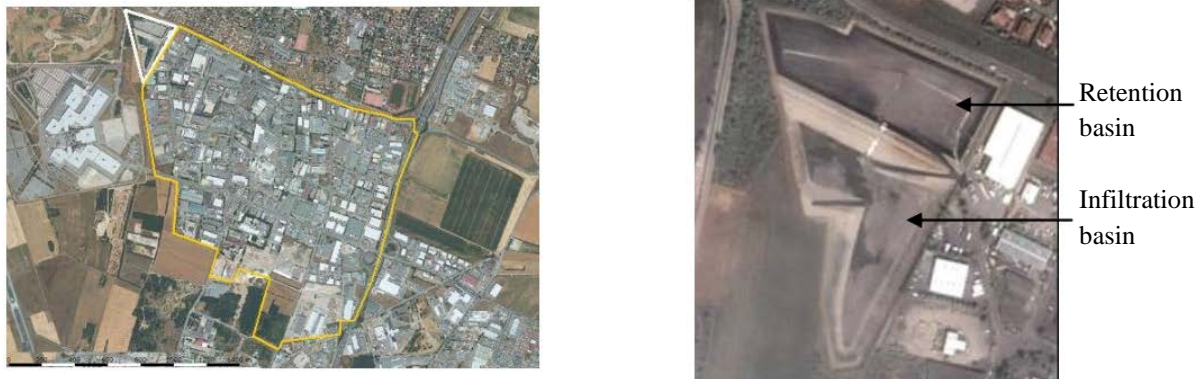
Figure 2. Aerial view of: the Chassieu catchment (left) (Source: www.othu.org) and the retention and infiltration basins (right) (source: Métadier, 2011).
