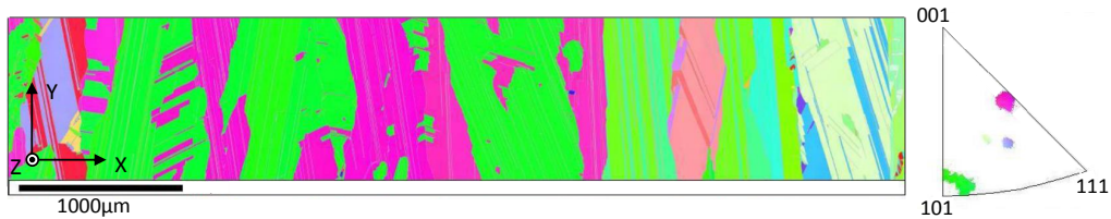
FIGURE 2.6: RST grain orientation distribution. Color coded map (left) where Y corresponds to the drawing direction. Inverse pole figure (right),
