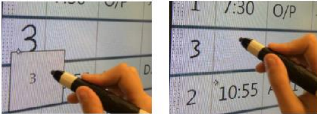
Figure 73. Writing recognition to change the OR number associated to a case.
