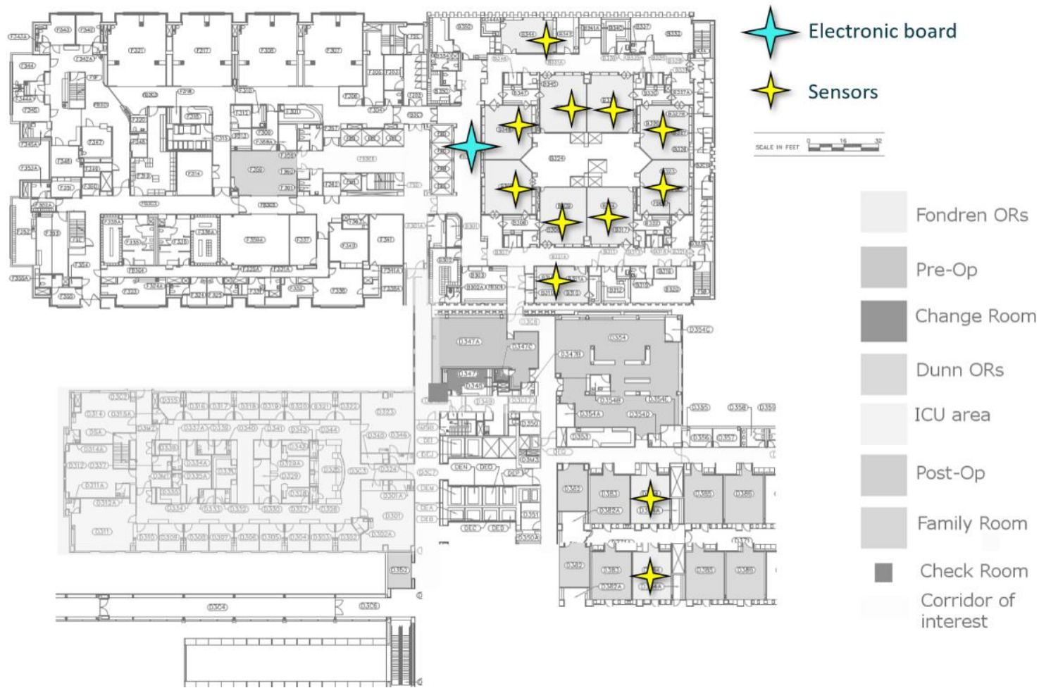
Figure 94. FondrenOR map and the placement of the OR sensors and OnBoard (Electronic Board).
