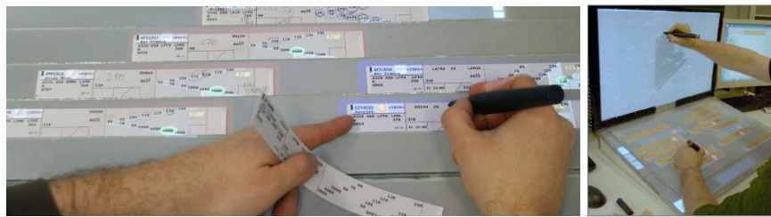
Figure 16. Strip'TIC: using augmented reality on tangible object to manage flights. On the right: two controllers using the Strip'TIC prototype (digital pens, augmented radar, stripboard, and paper strips).
