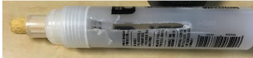
Figure 102. Pen enable to contain an embedded microcontroller. The pen was a little too small so we had to make a little cut on the side.
