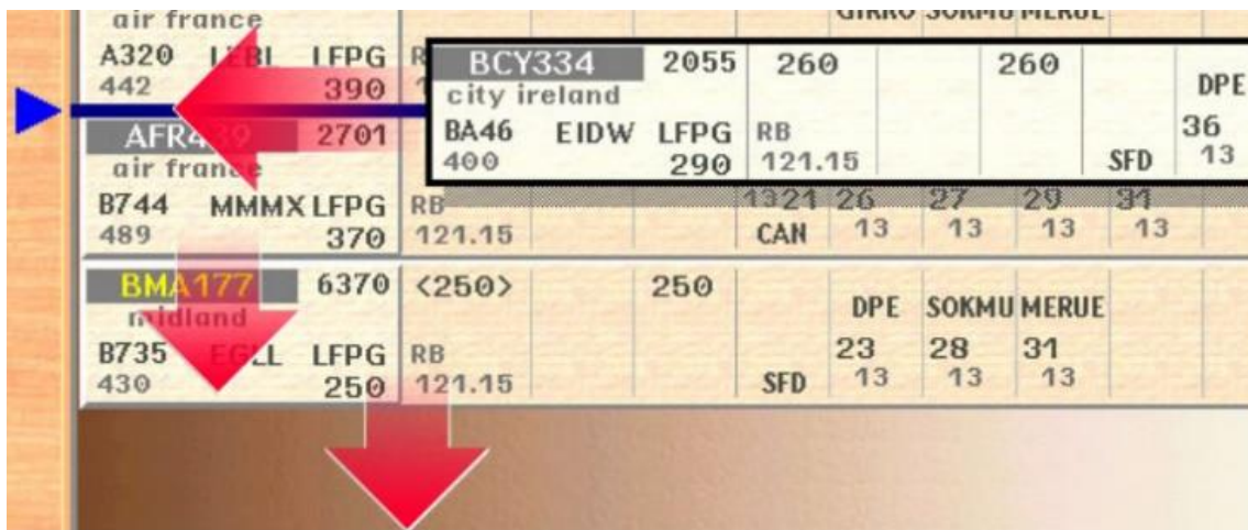
Figure 14. Digital strips visualization and manipulation offered by the Digistrip system.
