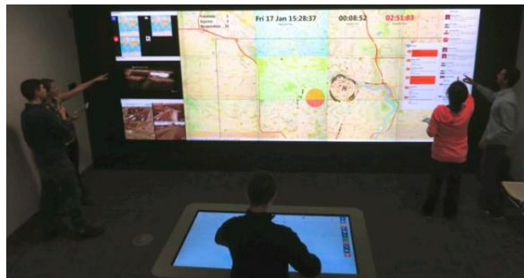
Figure 18. ePlan multi interfaces system, including at the back a large map visualization and at the front a multitouch table top interface. Photo credits: [45].
