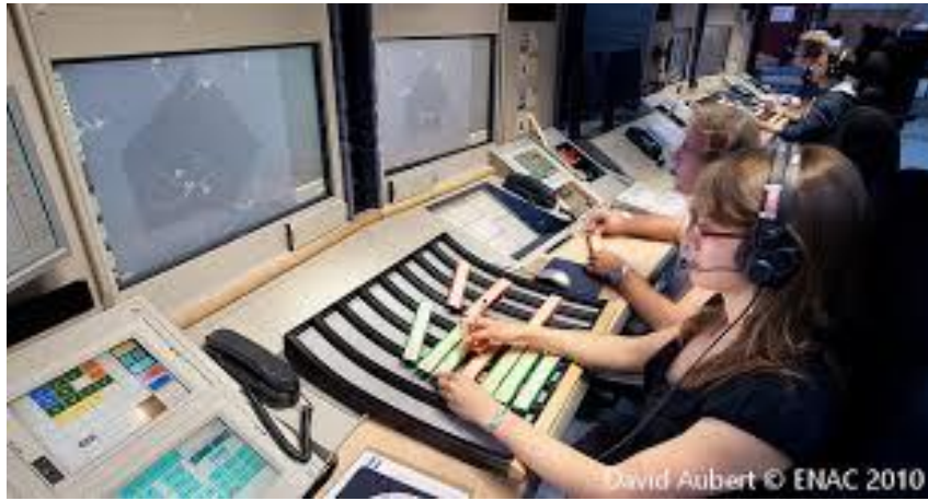
Figure 12. Example of an ATC workstation position and paper strips used in civil aviation to manage the flights.
