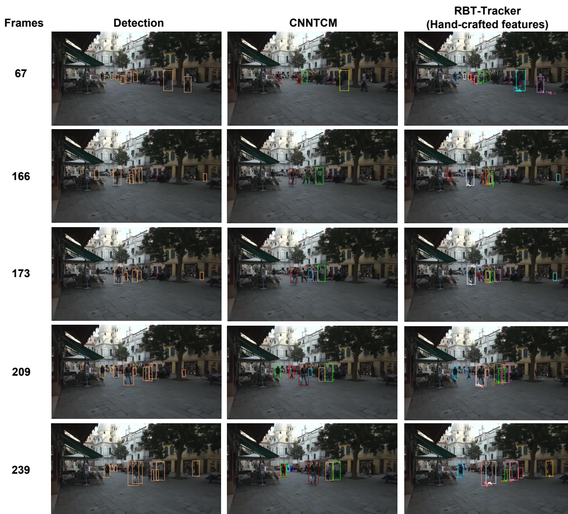
Figure 7.3: The noise filtering step of CNNTCM and RBT-Tracker (hand-crafted features) on Venice-1 sequence. The left to right columns are the detection, the tracking performance of CNNTCM and RBT-Tracker (hand-crafted features), respectively. The top to bottom rows are the scenes at frame 67, 166, 173, 209 and 239. RBT-Tracker (hand-crafted features) tries to track almost all detected objects in the scene while CNNTCM filters much more objects than RBT-Tracker (hand-crafted features) and manages to track these filtered objects in order to achieve better tracking performance. The more detections are filtered, the more false negatives (FN) increase. Therefore, CNNTCM has more false negatives than RBT-Tracker (hand-crafted features). On the other side, the illustration shows that the people detection results include a huge number of noise. Because of keeping more fake detected objects to track, tracking performance of RBT-Tracker (hand-crafted features) has more false positives than CNNTCM .
