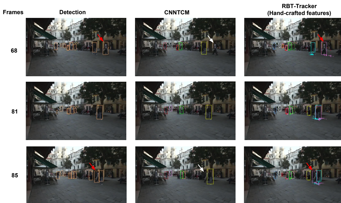
Figure 7.2: The illustration of the tracking performance of CNNTCM and RBT-Tracker (hand-crafted features) on sequence Venice-1 for the occlusion case. The left to right columns are the detection, the tracking performance of CNNTCM and RBT-Tracker (hand-crafted features) in order. The top to bottom rows are the scenes at frame 68, 81 and 85 which illustrate the scene before, during, and after occlusion, respectively. The tracker RBT-Tracker (hand-crafted features) tracks correctly the occluded objects (pointed by red arrows, marked by cyan and pink bounding-boxes). However, instead of tracking all occluded objects, tracker CNNTCM filters the occluded object (pointed by the white arrow) and track only the object (marked by the yellow bounding-box).
