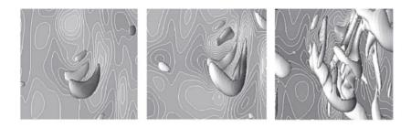
Fig. 2.15 Evolution of an hairpin vortex generated by a transitional natural convection flow. Structures are visualised using the *Q*-criterion. (Abramov et al., 2014)
