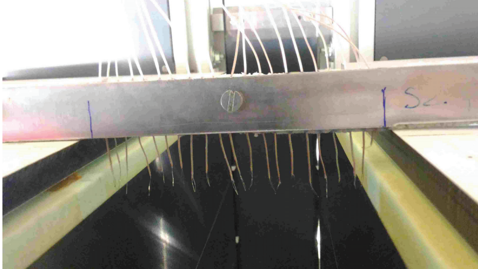
Fig. 3.3 Pictures of the outlet thermocouples
