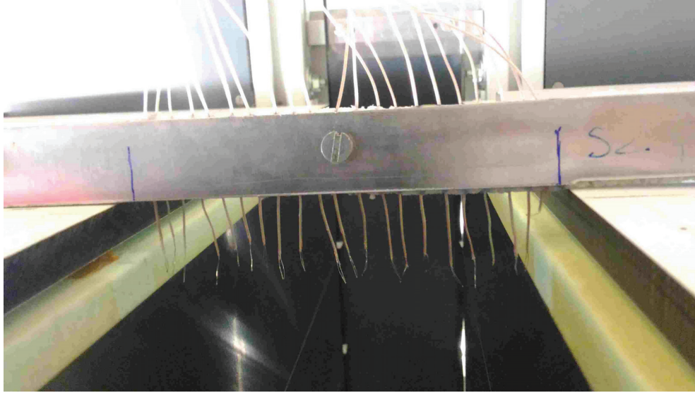
Fig. 3.3 Pictures of the outlet thermocouples
