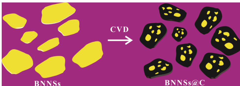
Fig. 5-1 Schematic illustration of the synthesis procedure of BNNSs@C hybrids
