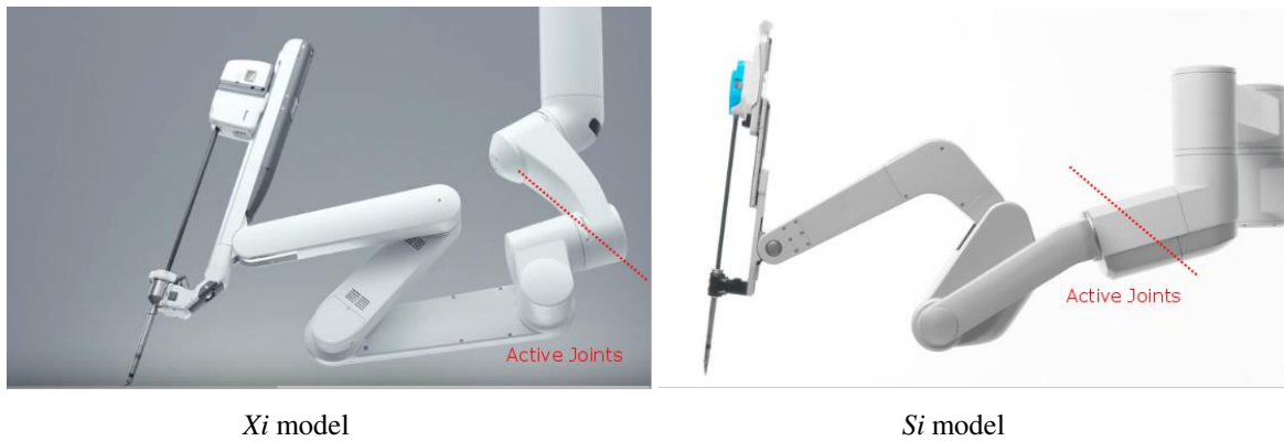
Figure 3.20 Actuated (active) joints in da Vinci robot
