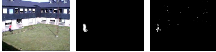
Figure I.6: On the left and at the middle are sample input and ground truth images respectively from the 2014 CDnet dataset, PTZ category. To the right is the image produced by SOM-QE on detecting the changes between the input image and its next image frame on the video. The PTZ category of images posed unique challenges on change detection, with other methods in the literature managing F1 score of less than 0.30. SOM-QE scored an F1 score of 0.39, which is the best score in this category.
