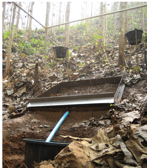
Fig 4.1: A) Rain simulation experiment under different land use. B) Example of rain simulation used under teak without understory (TWO). Runoff waters from the exit tube of the 1m 2 plot were determined every 30 sec using 100mL plastic bottle in order to calculate runoff volume during the rain simulation. Concomitantly with the runoff volume, samples were collected three times at T1, T2 and T3 during the rain simulation and a composite sample (CS) was collected from the bucket at the end of the rain simulation for measurement of dissolved organic carbon (DOC), colored dissolved organic matter (CDOM), Total suspended sediment (TSS) and total organic carbon (TOC) in TSS and bacterial functioning and diversity
