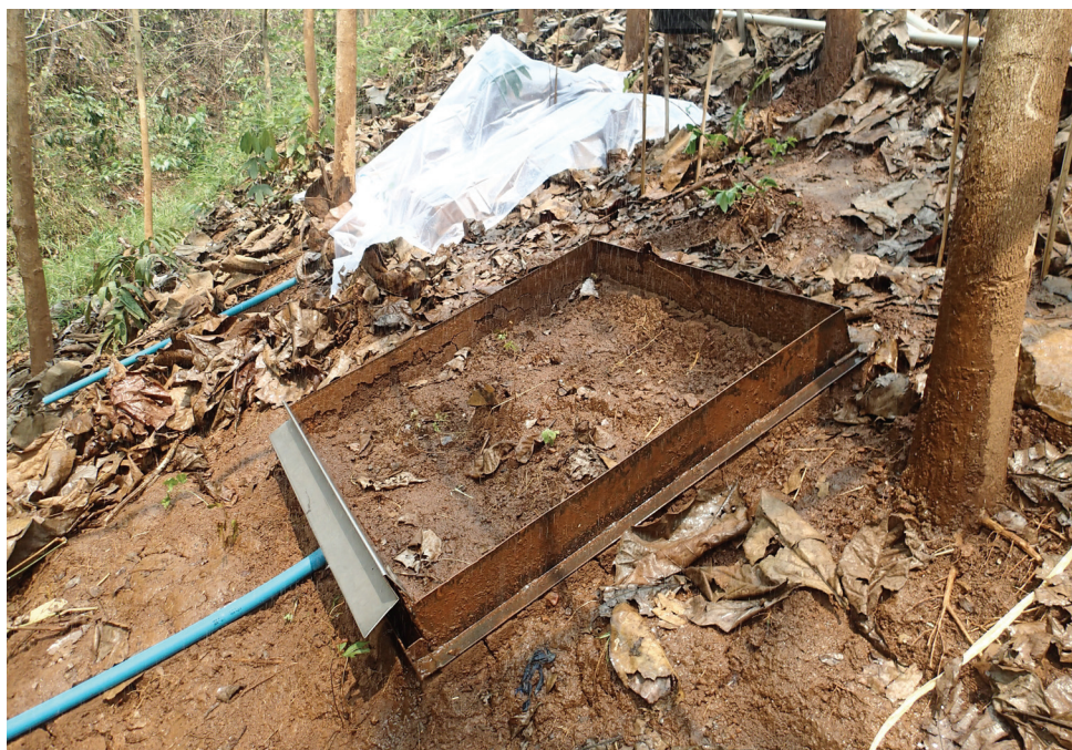
Fig 2.4: Rain simulation in the Houay Pano catchment, in the teak without understory (TWO) treatment
