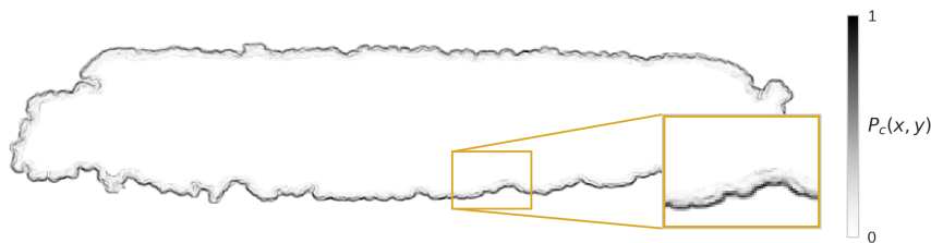
Figure 6.10 Contour probability P_c(x, y) obtained from P_s(x, y) . The result has been scaled in the 0-1 range.
