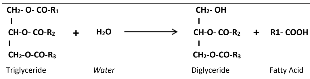
Figure 2-6. The typical hydrolysis reaction
