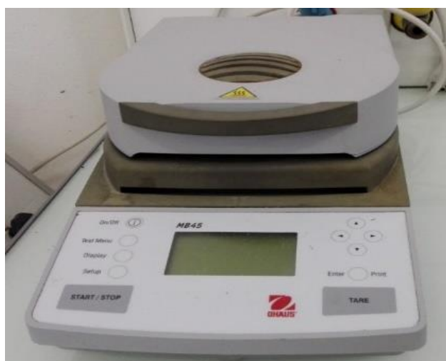
Figure 3-5. OHAUS MB45 Moisture Analyzer
