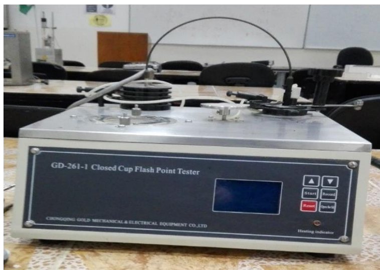
Figure 3-12. Pensky-Martens Closed Cup Flash Point Tester
