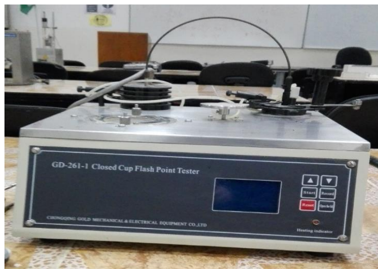
Figure 3-12. Pensky-Martens Closed Cup Flash Point Tester
