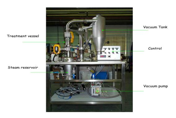
Figure 5-2. Lab-scale Instant controlled pressure drop (DIC) unit.
