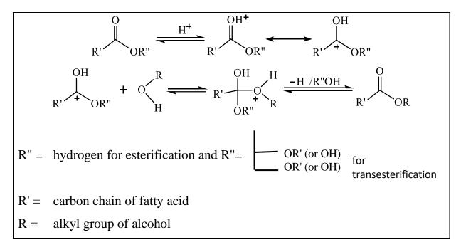
Figure 2-10. Mechanism for homogeneous acid catalysis in esterification and transesterification [230]
