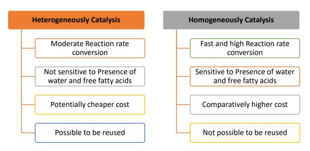
Figure 2-11. Comparison between homogeneous and heterogeneously catalyzed transesterification [229]
