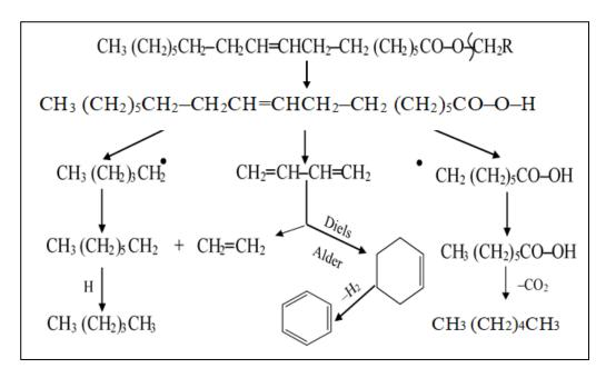
Figure 2-3. The mechanism of thermal decomposition of triglycerides [182]
