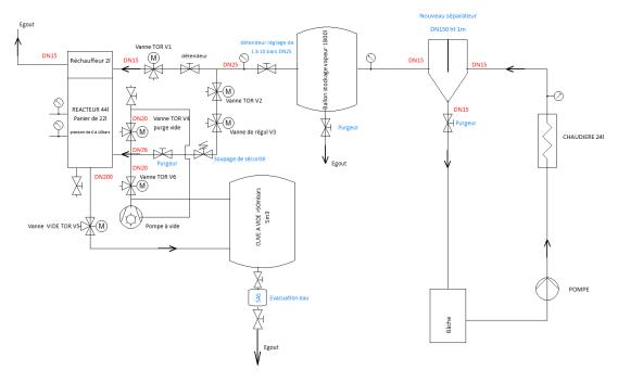
Figure 5-4. Instant controlled pressure drop (DIC) set-up
