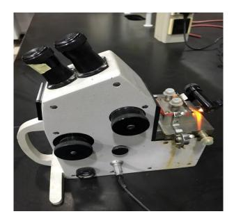
Figure 3-6. Abbe 60 refractometer
