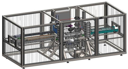
Figure 5-3. Instant controlled pressure drop (DIC) industrial unit
