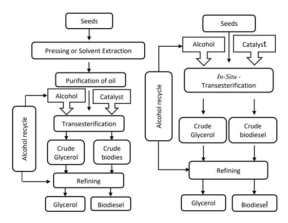
Figure 2-12. Comparison between transesterification and in-situ transesterification process
