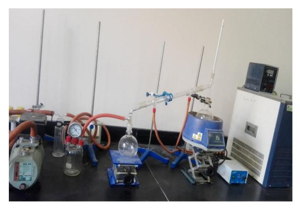
Figure 3-13. Vacuum Distillation Apparatus
