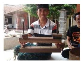
Figure 2.12: Wooden blades for clamping palm leaves
