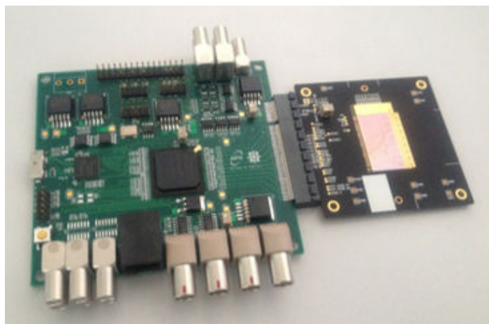
Figure 2.13 – DAQ read-out board connected an ALPIDE chip
