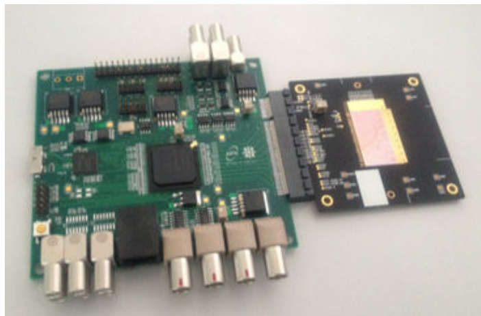
Figure 2.13 – DAQ read-out board connected an ALPIDE chip
