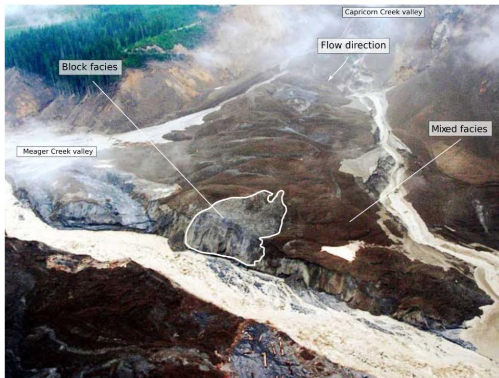
Figure B7. Helicopter view of the Meager barrier after the dam breach. Photo courtesy of D.B. Steers.
