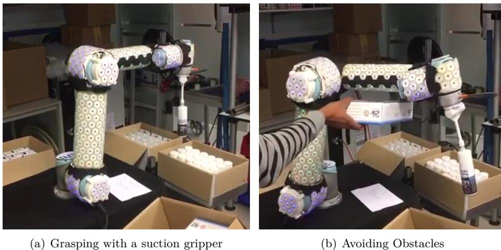
Figure 2.18: Illustrating obstacle avoidance while picking and placing small objects using a suction gripper. The full scenario video can be seen in this [video](#).
