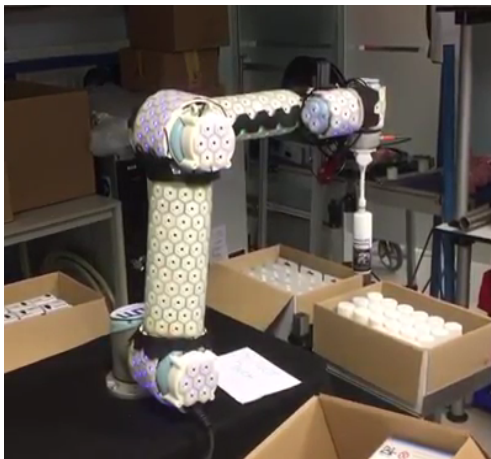
(a) Grasping with a suction gripper
