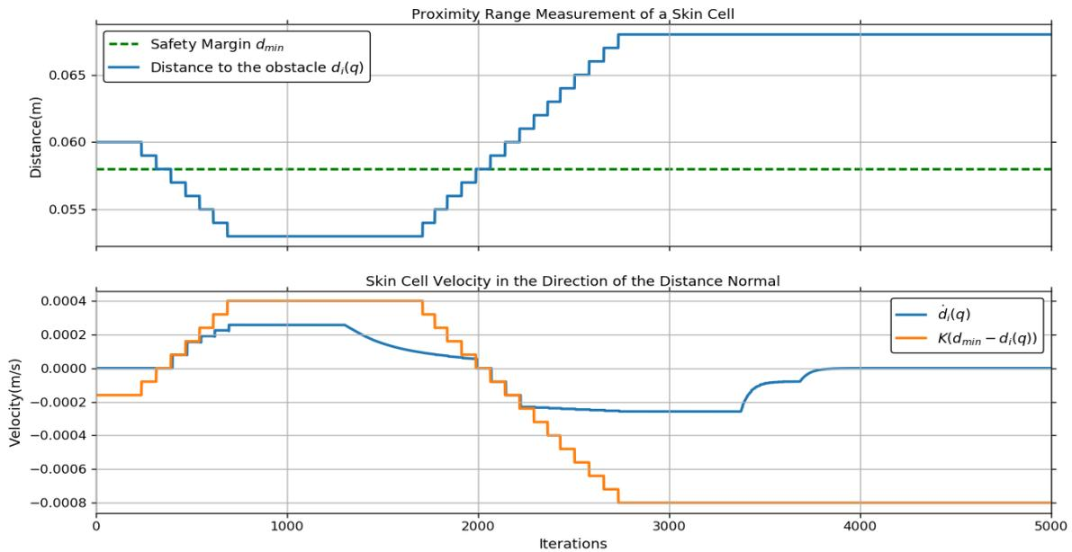
Figure 2.17: Plot showing the velocity of the skin cell  $i$ , when the other skin cells measure a distance of 6cm, which is just 2mm larger than the safety margin  $d_{min}$ . In this scenario, it is not possible to satisfy all the skin cell inequalities (2.10).
