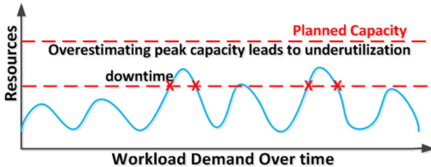
Figure 1.1 Resource over-/under-provisioning
