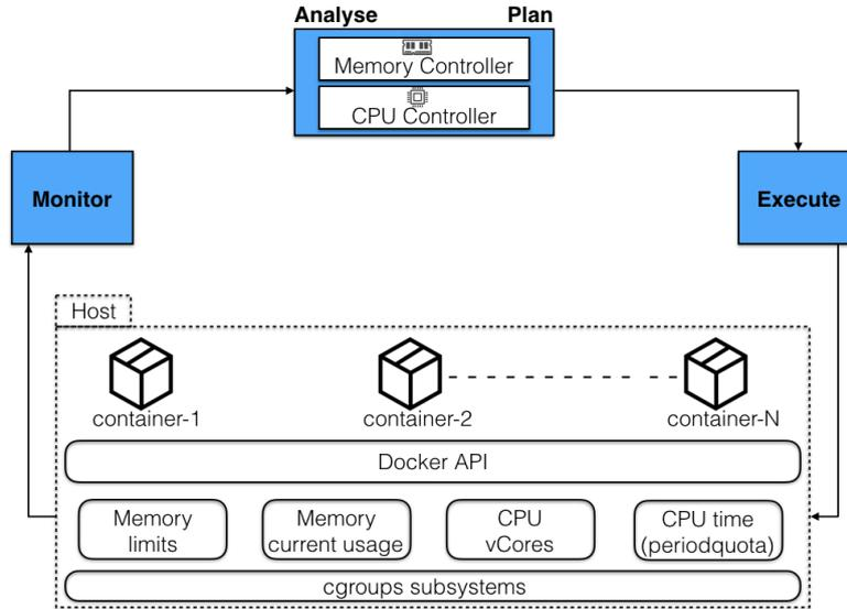
Figure 3.2 ELASTICDOCKER architecture
