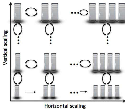
Figure 2.1 Horizontal vs vertical elasticity
