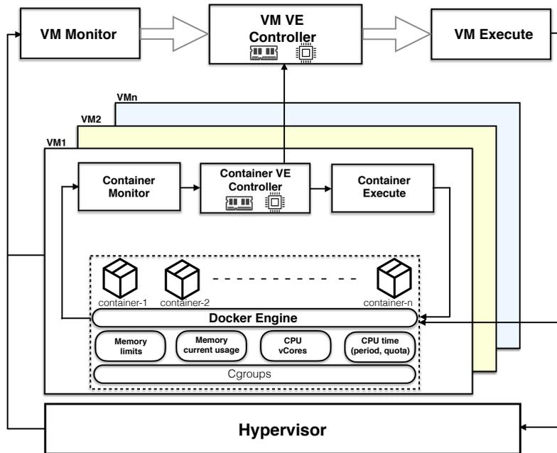
Figure 3.3 Coordinated elastic controllers between VMs and containers
