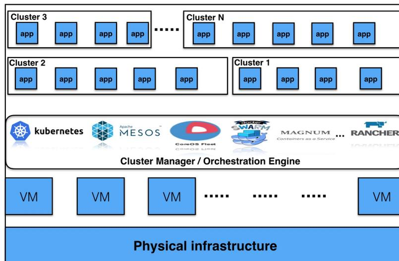
Figure 2.6 Container orchestration engines
