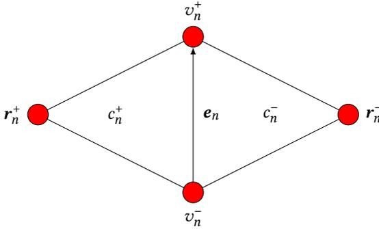
Fig. 4.1.: Definition of the RWG functions. The vector  $\mathbf{e}_n$  denotes the directed edge,  $c_n^+$  and  $c_n^-$  denote the domains of the cells,  $v_n^+$  and  $v_n^-$  denote vertices on the edge  $\mathbf{e}_n$ , and  $\mathbf{r}_n^+$  and  $\mathbf{r}_n^-$  are the vertices opposite to the edge  $\mathbf{e}_n$ .
