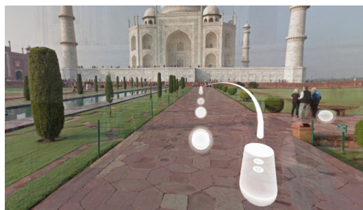
Figure 4.1: Example of viewpoint switching options appearing in a viewport in the Google Earth VR [57] interface, i.e., walk-through functionality. Each white sphere appearing in the viewport represents a viewpoint that the user can switch to. The viewpoint switch can be selected using a controller, whose virtual representation is appearing in the viewport as well.
