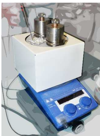
Figure 50: Autoclave reactors placed inside a pre-heated isothermal device on a hotplate
