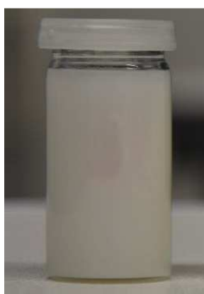
Figure 51: Synthesized suspension of zirconia after solvothermal reaction.
