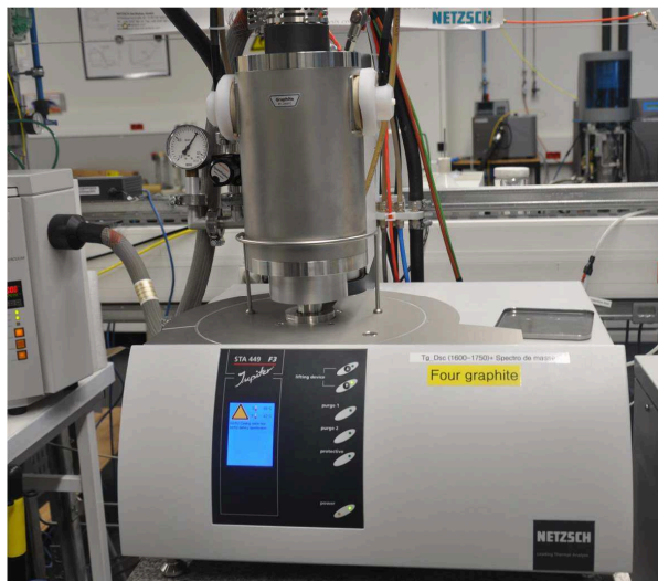
Figure 54: TGA device used for characterization (TGA NETZSCH STA 449 F3 Jupiter)
