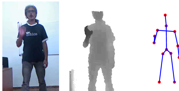
Figure 1.1 – Sample colour frame, depth map and body pose coordinates as returned by a kinect camera in the Montalbano v2 dataset [Escalera et al., 2014].
