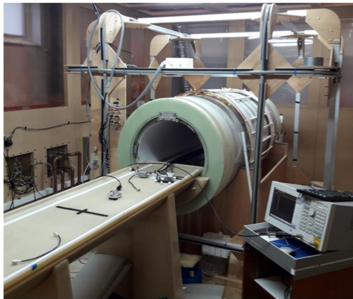
Figure 0-1 : IRM à champ cyclé de 0.2 T (School of Medicine, Medical Sciences and Nutrition, University of Aberdeen, UK).
