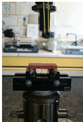
FIGURE 3.2.3 – Montage de flexion 3points
