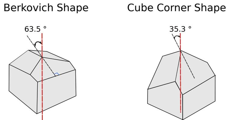
FIGURE 2.5: Berkovich and cube corner indenter tip geometries
