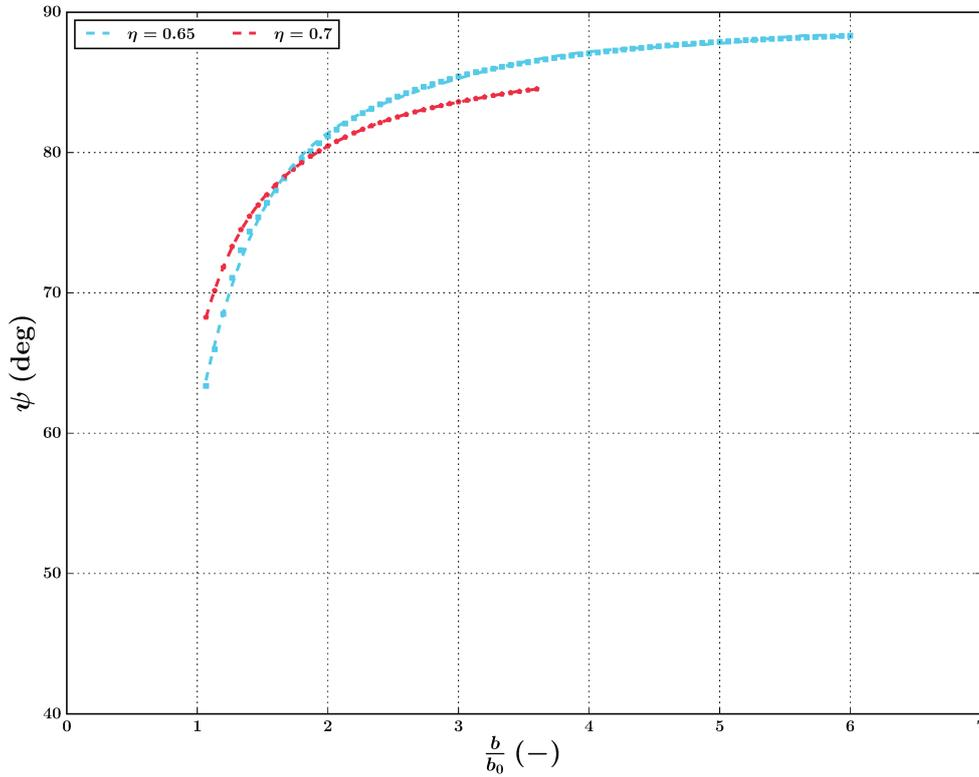
FIGURE 4.7: Mode mixity angle  $\psi$  as a function of the normalized position of the crack front  $\frac{b}{b_0}$ , where  $b$  is the half width of the blister and  $b_0$  the half width of the initial defect.
