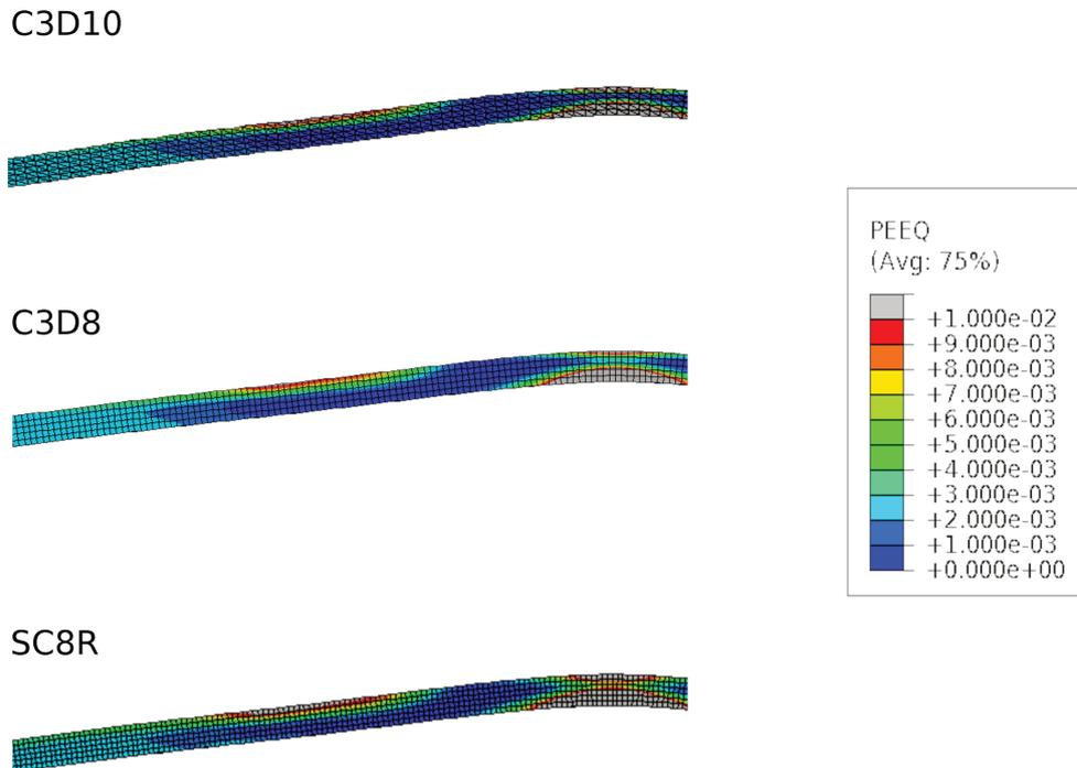
FIGURE 4.10: Equivalent plastic strain mapping obtained using quadratic tetrahedrons (C3D10), linear bricks (C3D8) and linear shell elements (SC8R) in the frame of explicit integration scheme.
