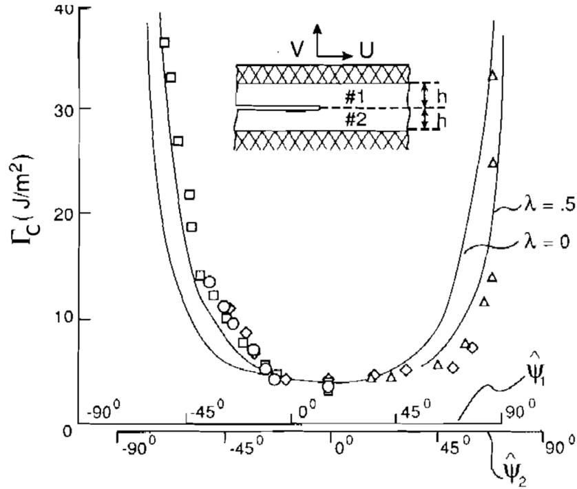
FIGURE 1.8: Data from [65] for an epoxy #1 / glass #2 interface:  $\psi_1$  axis is obtained using  $l_1 = 12,7\text{mm}$  and  $\psi_2$  using  $l_2 = 127\mu\text{m}$ . The solid curves represent  $G_c(\psi_2)$  as given by equation 1.35
