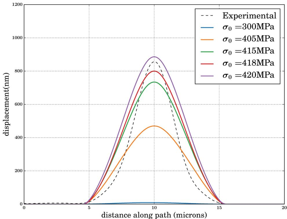
FIGURE 3.23: Comparison between the experimental blister's profile and elastic-plastic numerical model results in the case of straight blister (Ludwik strain hardening  $\sigma_y = 400$  MPa,  $K = 50$  MPa,  $n = 0.25$ ) for different  $\sigma_0$  values
