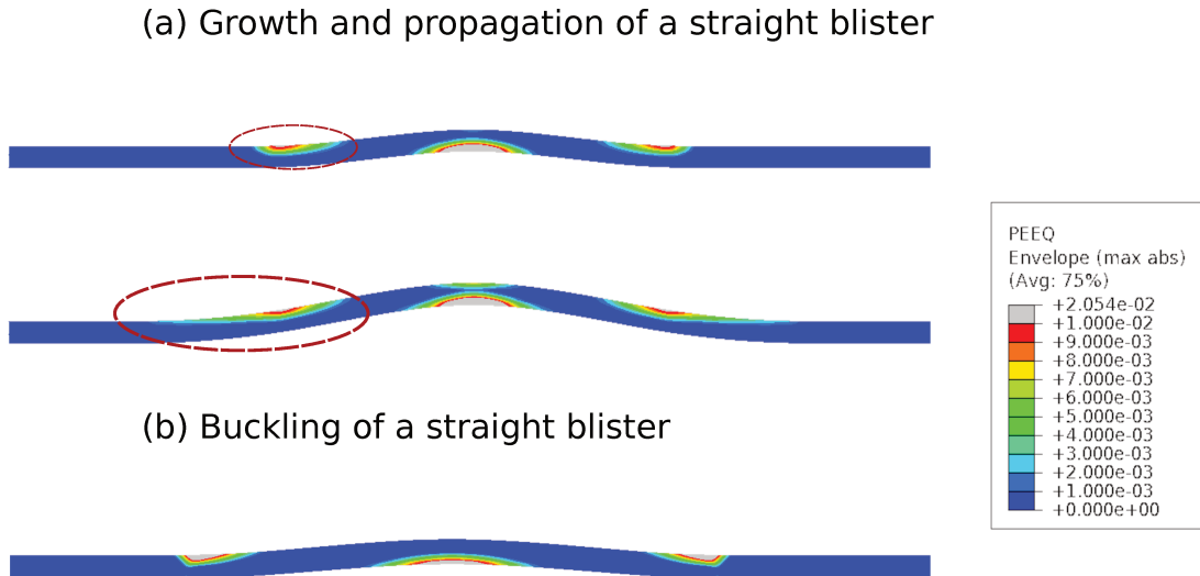
FIGURE 4.13: Equivalent plastic deformation mapping in the cases of pure buckling (a) and buckling-driven delamination (b). Both results were obtained for the same load and elastic plastic behaviour. We have \sigma_0 = \sigma_y = 700 . The remaining parameters are detailed in table 4.4.
