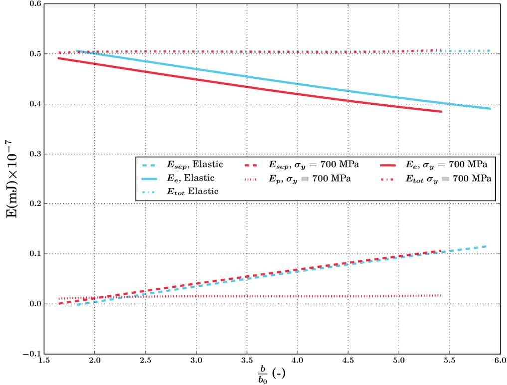
FIGURE 4.14: Energy as a function of the normalized position of the crack front  $\frac{b}{b_0}$ , where  $b$  is the half width of the blister during propagation and  $b_0$  the half width of the initial defect.  $E_e$  represents the elastic energy,  $E_p$  the plastic energy and  $E_{sep}$  the energy used to fracture the interface. The figure features two cases: purely elastic thin film ( $\sigma_0 = 700$  MPa) and elastic-plastic thin film ( $\sigma_0 = \sigma_y = 700$  MPa).
