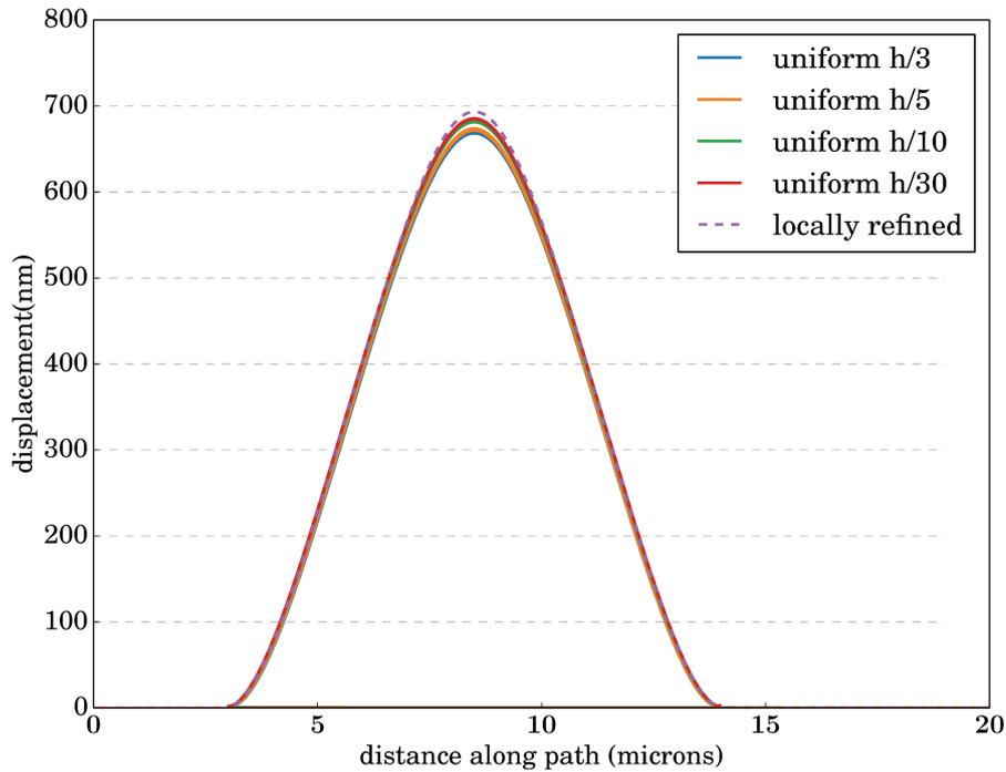
FIGURE A.4: *Effect of mesh refinement on the buckling profile of straight blisters. The profiles are obtained for the same ratio  $\frac{\sigma_0}{\sigma_y} = 1.03$ , the same hardening law (Ludwik  $\sigma_y = 800$  MPa,  $K = 130$  MPa,  $n = 0.25$ ) and different solid element sizes. (see figure A.5)*
