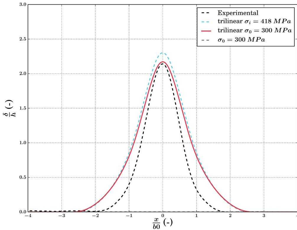
FIGURE 4.21: *Effect of non-monotonic loading on elastic-plastic buckling-driven delamination in the case of straight blister (Ludwik strain hardening  $\sigma_y = 400$  MPa,  $K = 50$  MPa,  $n = 0.25$ )*
