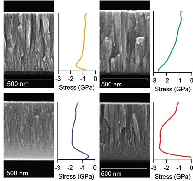
FIGURE 3.21: FEG-SEM images showing the influence of substrate potential and oxygen doping on the microstructure of molybdenum thin films. Top left: Mo at floating potential, top right: Mo at  $-75$  V, bottom left: Mo with 2 sccm of  $O_2$  at floating potential and bottom right: Mo with 2 sccm of  $O_2$  at  $-75$  V. [29]
