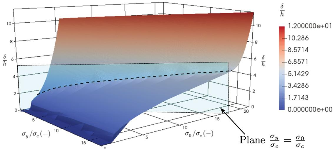
FIGURE 3.13: 3D representation of the normalized deflection  $\frac{\delta}{h}$  as function of  $\frac{\sigma_y}{\sigma_c}$  and  $\frac{\sigma_0}{\sigma_c}$ . This curve is plotted using the following Ludwik hardening:  $K = 500$  MPa and  $n = 0.25$ .
