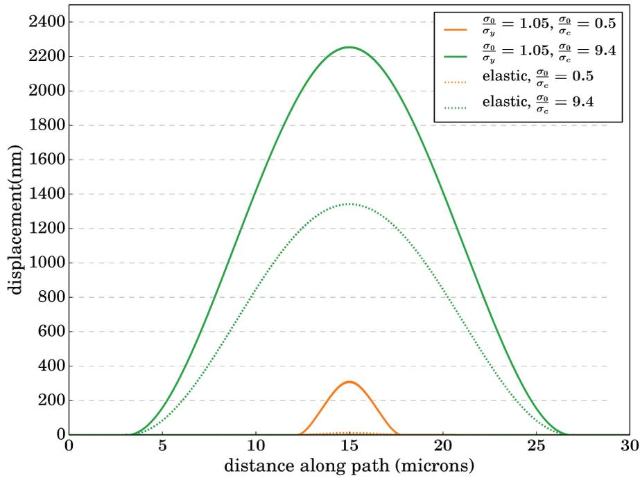
FIGURE 3.10: Comparison between elastic and elastic plastic (Ludwik  $\sigma_y = 800$  MPa,  $K = 130$  MPa,  $n = 0.25$ ) profiles for  $\frac{\sigma_0}{\sigma_c} = 0.5$  and  $\frac{\sigma_0}{\sigma_c} = 9.4$ .
