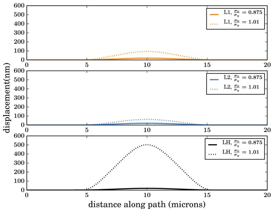
FIGURE 3.18: Straight blisters' profiles for different elastic-plastic behaviours: L1 (Ludwik:  $\sigma_y = 400$  MPa,  $K = 50$  MPa,  $n = 0.25$ ), L2: (Ludwik:  $\sigma_y = 400$  MPa,  $K = 130$  MPa,  $n = 0.25$ ), LH (Linear hardening:  $\sigma_y = 400$  MPa,  $K = 80$  MPa)
