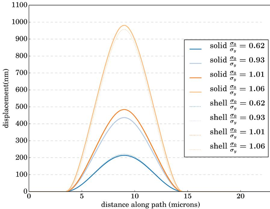
FIGURE A.2: Effect of the element's type (solid or shell elements) on the elastic-plastic buckling of straight blister. The profiles obtained are given for different  $\sigma_0$  and the same hardening law (Ludwik  $\sigma_y = 800$  MPa,  $K = 130$  MPa,  $n = 0.25$ )
