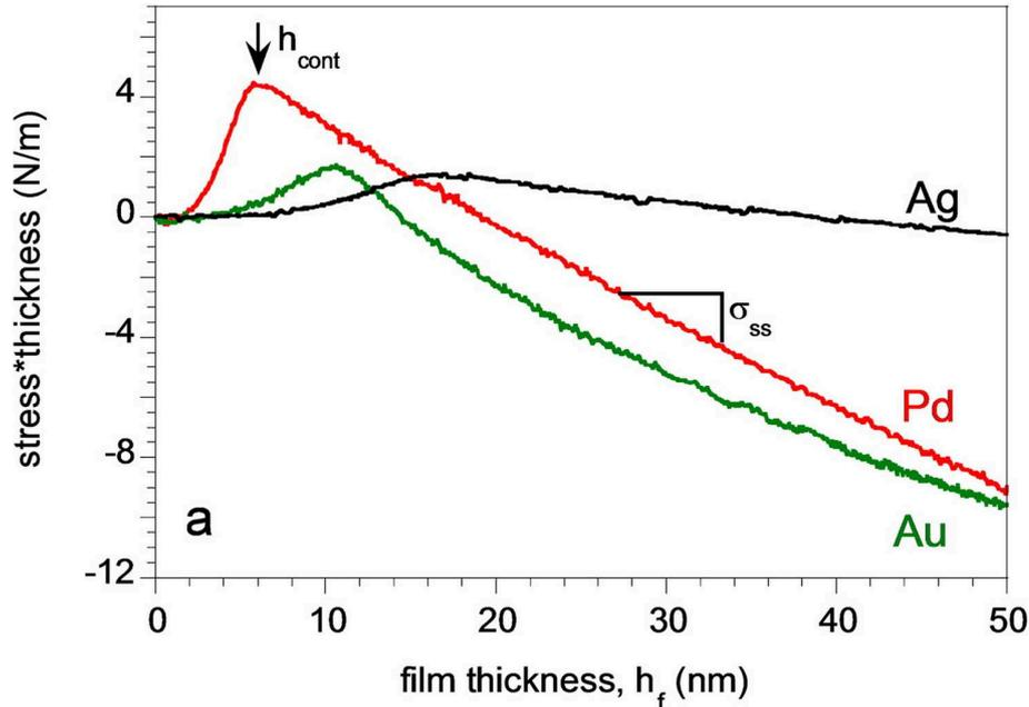
FIGURE 3.20: Film force evolution during sputter deposition of Ag, Au and Pd films on a-SiOx. The film thickness corresponding to the tensile peak is referred as  $h_{cont}$  [1].
