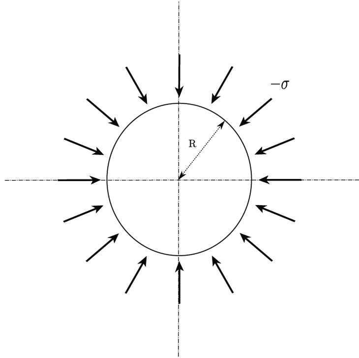
FIGURE 1.2: Geometry and conventions of the circular blister.
