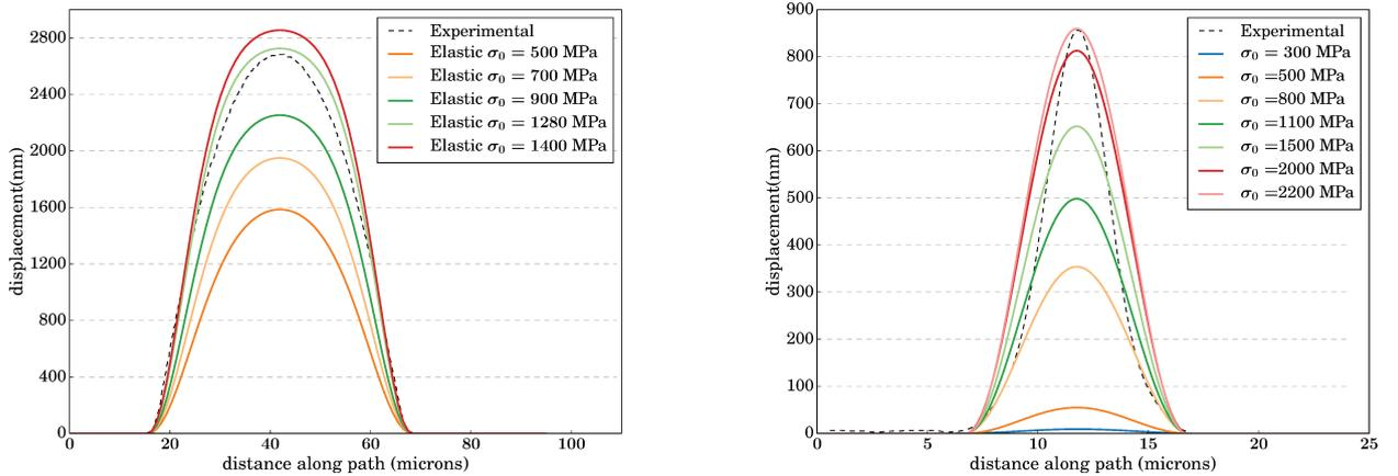
FIGURE 3.4: Comparison between the experimental profiles of circular (left) and straight (right) buckles with results of FEM simulations assuming a linear elastic behavior of the film, obtained for several values of  $\sigma_0$ .
