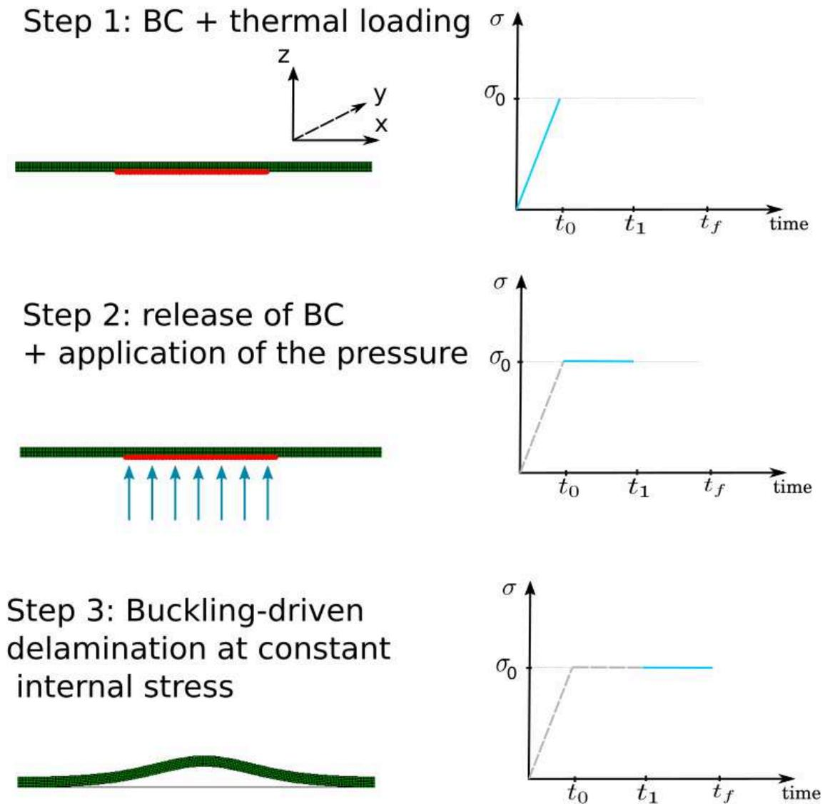
FIGURE 4.22: Scheme of the steps applied to ensure the occurrence of buckling-driven delamination at constant load  $\sigma_0$ . In the first step, the bottom nodes of the defect area of the film are blocked along the  $z$  - axis and the thermal loading of the film is performed. In the 2<sup>nd</sup> step, the defect nodes are released and a small pressure is applied to trigger buckling. In the final step, buckling-driven delamination occurs at constant loading.
