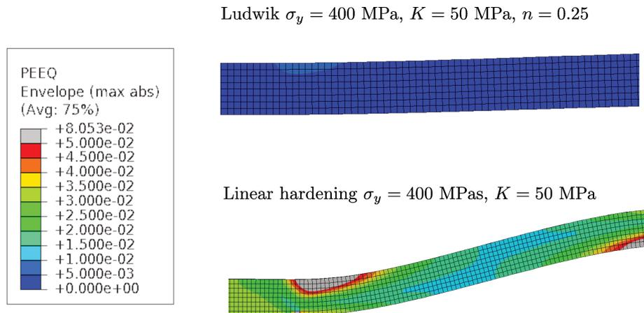
FIGURE 3.17: Effect of the hardening law on plastic strain at the base of straight blisters ( $\sigma_0 = 404$  MPa)
