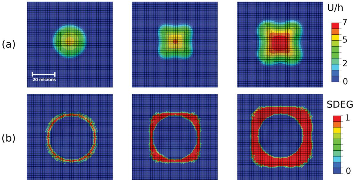
FIGURE 4.25: Various stages of growth of a circular defect submitted to constant loading  $\sigma_0$ . The row (a) features the evolution of the normalized out-of-plane displacement  $\frac{U}{h}$  and the row (b) shows the corresponding degradation variable of the interface SDEG. SDEG=0 means that the interface is intact, SDEG=1 means that the fracture is completed and intermediate SDEG values corresponding to an ongoing fracture process.
