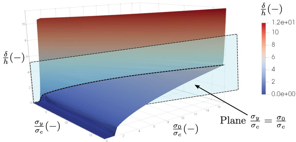
FIGURE 3.11: 3D representation of the normalized deflection  $\frac{\delta}{h}$  as function of  $\frac{\sigma_y}{\sigma_c}$  and  $\frac{\sigma_0}{\sigma_c}$ . This curve is plotted using the following Ludwik hardening:  $K = 130$  MPa and  $n = 0.25$ .
