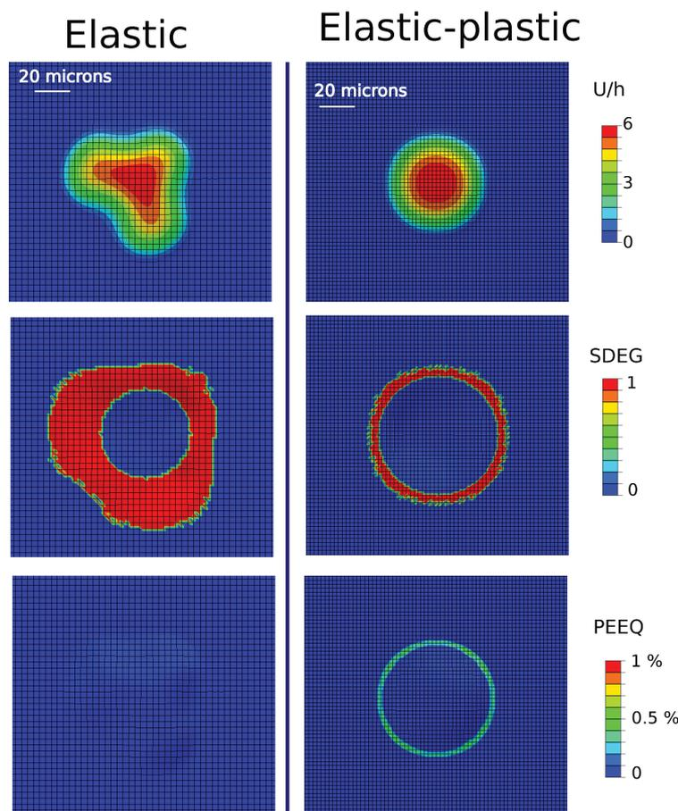
FIGURE 4.28: Various stages of growth of a circular blister submitted to constant load  $\sigma_0$  in the case of an elastic and an elastic-plastic behaviour ( $\sigma_y = 800 \text{ MPa}$ ,  $K = 50 \text{ MPa}$ ,  $n = 0.25$ ). Each case features the mapping of the normalized out-of-plane displacement  $\frac{U}{h}$  at the equilibrium point, the corresponding degradation variable of the interface SDEG and the distribution of the plastic deformation.
