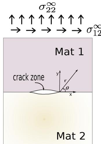
FIGURE 1.5: *Crack at an interface between two materials*
