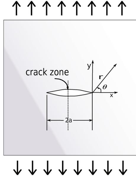
FIGURE 1.7: Conventions at crack tip in homogeneous material
