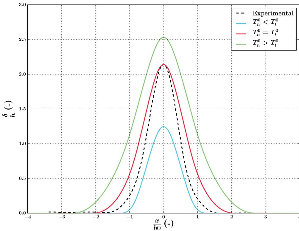
FIGURE 4.18: Comparison between the profiles obtained for different values of maximum normal and shear stress  $T_n^0$  and  $T_t^0$ . The cases  $T_n^0 < T_t^0$ ,  $T_n^0 = T_t^0$  and  $T_n^0 > T_t^0$  correspond respectively to the following couples  $(T_n^0, T_t^0)$ : (60, 120), (60, 60) and (60, 40) MPa
