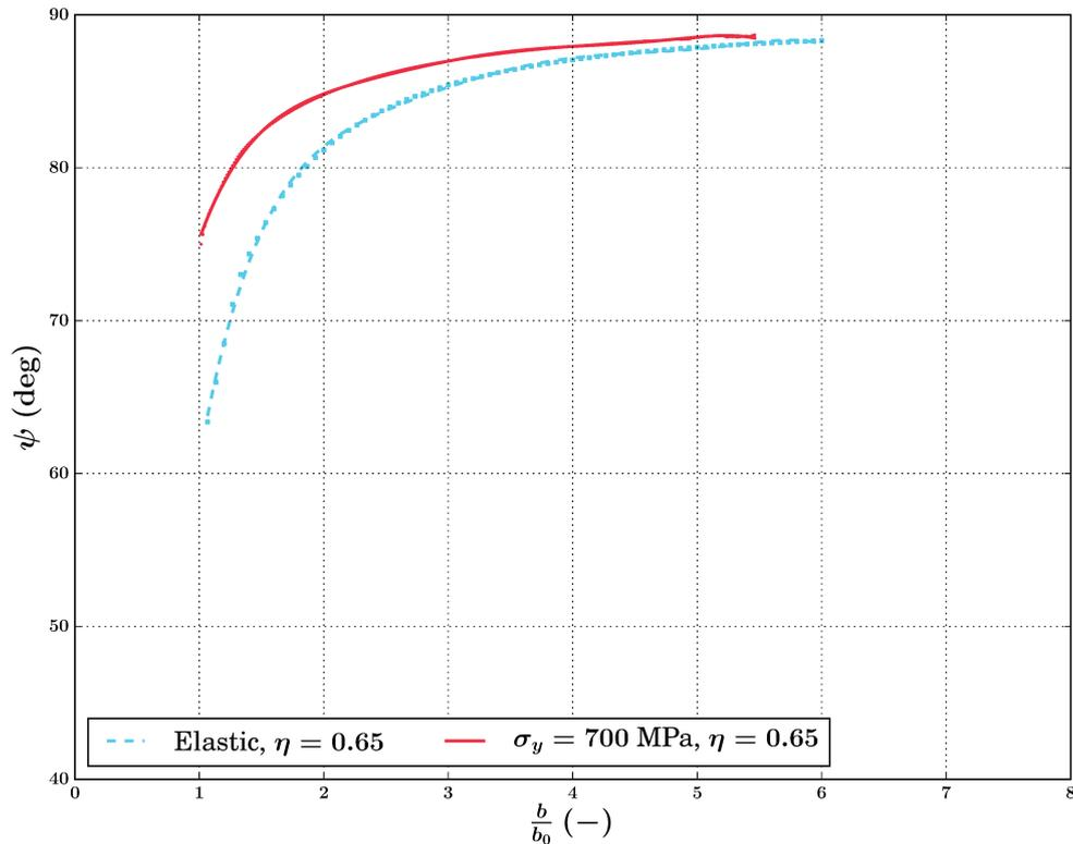
FIGURE 4.15: Mode mixity angle  $\psi$  as a function of the normalized position of the crack front  $\frac{b}{b_0}$ , where  $b$  is the half width of the blister and  $b_0$  the half width of the initial defect in the case of an elastic and an elastic-plastic response of the film.
