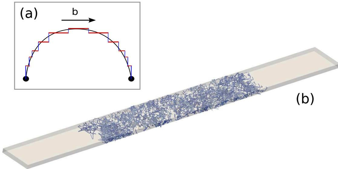
FIGURE 4.30: (a) Edge-screw discretization of a dislocation line. Blue lines are edge dislocations and red lines are screw dislocations. (b) Coupling finite element method with discrete dislocation dynamics. The Frank–Read sources are distributed randomly in a rectangular single crystal that represents the thin film. Different colours represent different slip systems.
