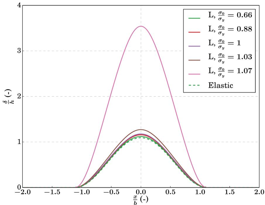
FIGURE 3.5: Comparison between elastic and elastic-plastic straight blisters' profiles. The y-axis represents normalized deflection  $\frac{\delta}{h}$ , where  $\delta$  is the out-of-plane displacement of the film and  $h$  the thickness of the film (fixed). All cases are subject to the same residual stresses ( $\sigma_0 = 800$  MPa). The elastic-plastic behaviour is described by Ludwik hardening with the following fixed parameters  $K = 130$  MPa,  $n = 0.25$ .
