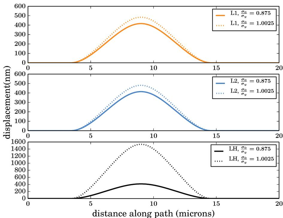
FIGURE 3.15: Straight blisters' profiles for different elastic-plastic behaviours: L1 (Ludwik:  $\sigma_y = 800$  MPa,  $K = 50$  MPa,  $n = 0.25$ ), L2: (Ludwik:  $\sigma_y = 800$  MPa,  $K = 130$  MPa,  $n = 0.25$ ), LH (Linear hardening:  $\sigma_y = 800$  MPa,  $K = 80$  MPa)
