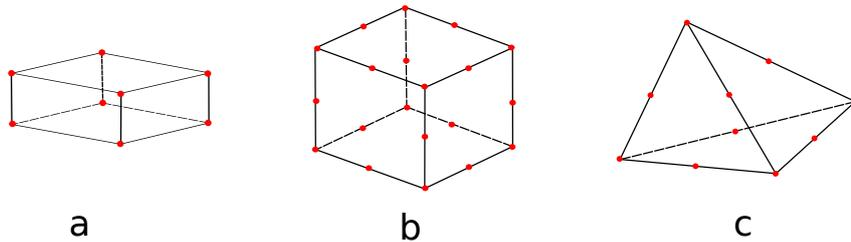
FIGURE A.1: *Shell and solid elements: (a) Continuum shell linear elements (8-node brick, SC8R), (b) Solid quadratic element (20-node brick, C3D20), (c) Solid quadratic element (10-node tetrahedron, C3D10)*
