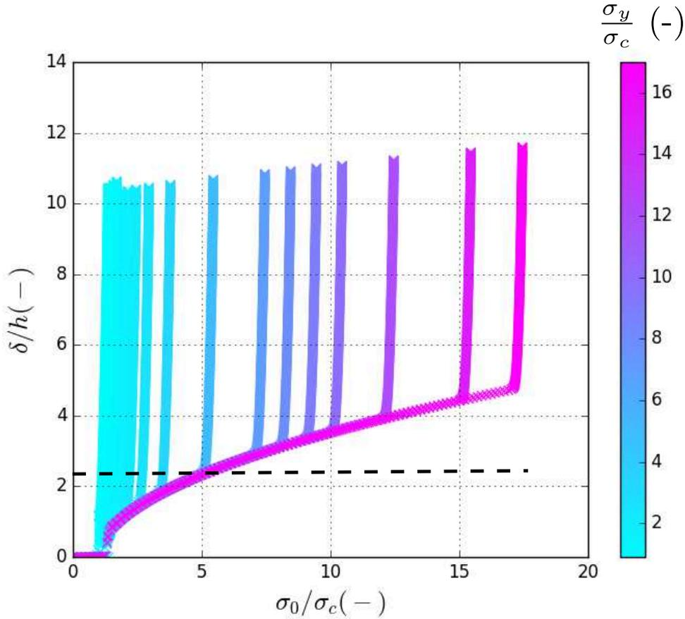
FIGURE 3.12: 2D projection of normalized deflection  $\frac{\delta}{h}$  as function of  $\frac{\sigma_0}{\sigma_c}$ . The graph features different level lines of  $\frac{\sigma_y}{\sigma_c}$ . These curves are plotted for a Ludwik hardening:  $K = 130$  MPa and  $n = 0.25$ .
