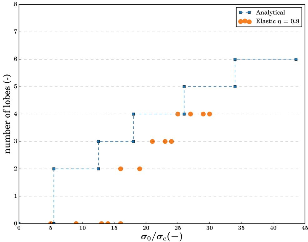
FIGURE 4.26: Number of lobes  $n$  resulting from the destabilization process of an initially circular blister at different loading ratios  $\frac{\sigma_0}{\sigma_c}$ . Numerical results are obtained using cohesive zone model for a mode mixity dependence parameter  $\eta = 0.9$  and Poisson's ratio of the film  $\nu = 0.44$ . The analytical results are obtained for  $\eta = 1$  and  $\nu = \frac{1}{3}$ .
