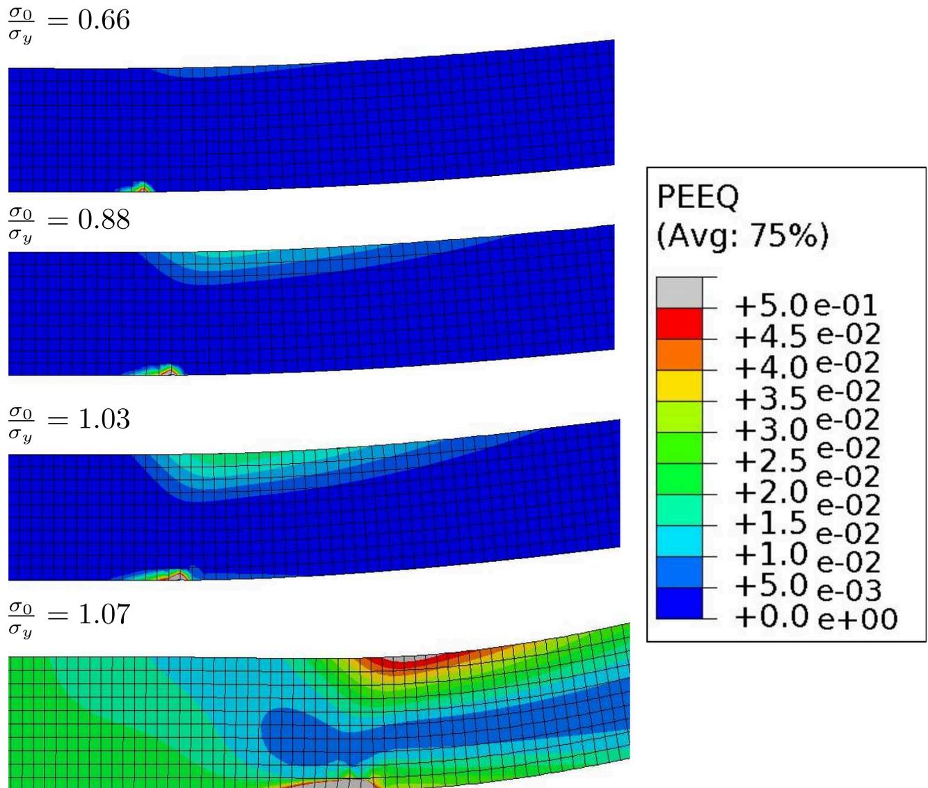
FIGURE 3.6: Equivalent plastic strain mapping for the cases  $\frac{\sigma_0}{\sigma_y} = 0.66$ ,  $\frac{\sigma_0}{\sigma_y} = 0.88$  and  $\frac{\sigma_0}{\sigma_y} = 1.03$ . All cases are subject to the same residual stresses ( $\sigma_0 = 800$  MPa). The elastic-plastic behaviour is described by Ludwik hardening with the following fixed parameters  $K = 130$  MPa,  $n = 0.25$ . We vary  $\sigma_y$
