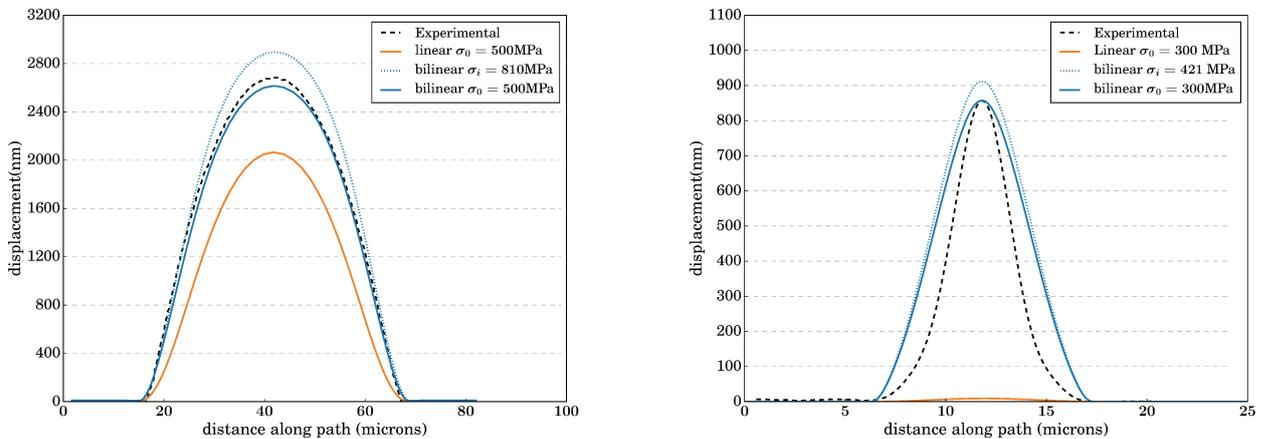
FIGURE 3.25: Effect of non-monotonic loading on elastic-plastic buckling in the case of circular blister (left  $\sigma_y = 800$  MPa) and straight blister (right  $\sigma_y = 400$  MPa) (Ludwik strain hardening  $K = 50$  MPa,  $n = 0.25$ )
