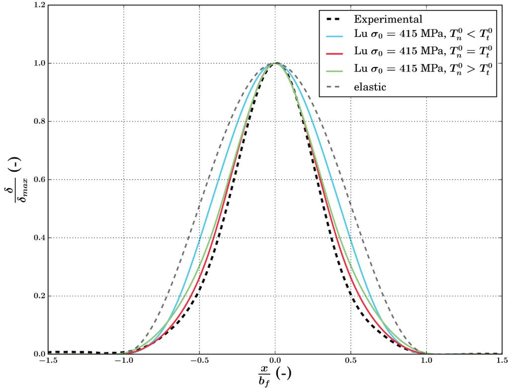
FIGURE 4.19: Normalized out-of-plane displacement  $\frac{\delta}{\delta_{max}}$  as a function of  $\frac{x}{b_f}$  for  $\sigma_0 = 415$  MPa,  $\sigma_y = 400$  MPa and for different values of  $(T_n^0, T_t^0)$ : (60, 120), (60, 60) and (60, 40) MPa.
