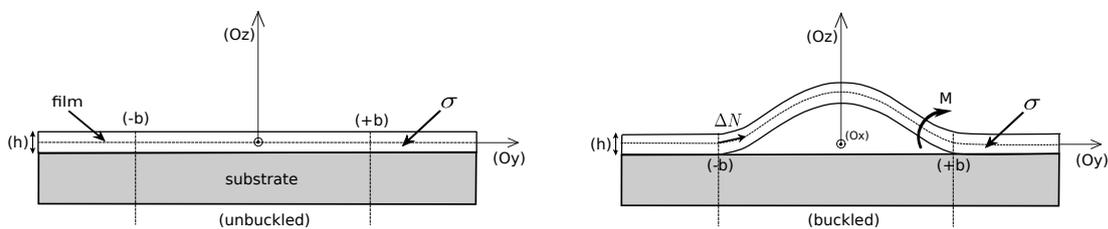
FIGURE 1.1: Geometry and conventions of the one-dimensional blister.  $\Delta N$  and  $M$  are respectively the resultant stress and the bending moment. left: unbuckled state; right: buckled state and local loading on the film.
