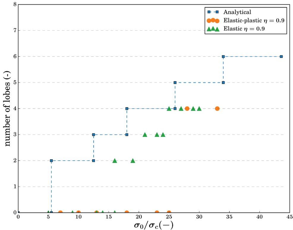
FIGURE 4.29: Number of lobes  $n$  resulting from the destabilization process of an initially circular blister at different loading ratios  $\frac{\sigma_0}{\sigma_c}$  for an elastic and an elastic-plastic thin film. Numerical results are obtained using cohesive zone model for a mode mixity dependence parameters of 0.9 and Poisson's ratio of the film  $\nu = 0.44$ .
