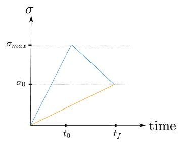
FIGURE 3.24: Different loading histories: Linear loading (orange) and bi-linear loading (blue).
