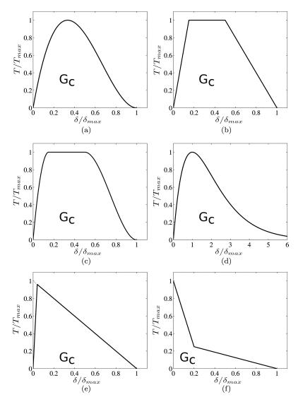
FIGURE 1.11: Example of traction-separation laws: (a) cubic polynomial, (b) trapezoidal, (c) smooth trapezoidal, (d)exponential, (e) linear softening, a,d (f) bilinear softening. from [77]
