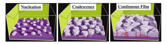
FIGURE 3.19: The regimes of microstructural evolution during Volmer-Weber film growth. [35]
