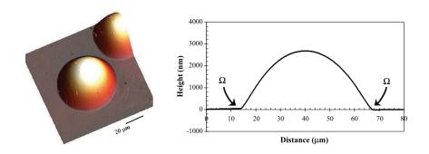
Figure 2.4: Buckling structure observed in gold film,  $630\,\mathrm{nm}$  thick, deposited on silicon substrate. A marked bending  $\Omega$  of the buckling structure is observed at the base of the circular blister. [18]
