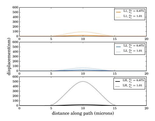
FIGURE 3.18: Straight blisters' profiles for different elastic-plastic behaviours: L1 (Ludwik: $\sigma_y = 400$  MPa, K = 50 MPa, n = 0.25), L2: (Ludwik: $\sigma_y = 400$  MPa, K = 130 MPa, K
