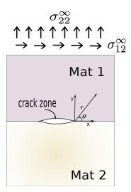
FIGURE 1.5: Crack at an interface between two materials
