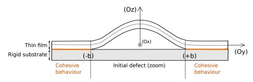
FIGURE 4.1: Mechanical model of buckling-driven delamination of thin film on rigid substrate.
