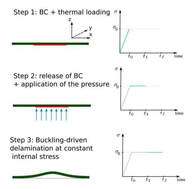
FIGURE 4.22: Scheme of the steps applied to ensure the occurrence of buckling-driven delamination at constant load  $\sigma_0$ . In the first step, the bottom nodes of the defect area of the film are blocked along the z-axis and the thermal loading of the film is performed. In the  $2^{nd}$  step, the defect nodes are released and a small pressure is applied ton trigger buckling. In the final step, buckling-driven delamination occurs at constant loading.
