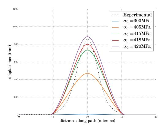
FIGURE 3.23: Comparison between the experimental blister's profile and elastic-plastic numerical model results in the case of straight blister (Ludwik strain hardening  $\sigma_v = 400 \text{ MPa}$ , K = 50 MPa, n = 0.25) for different  $\sigma_0$  values
