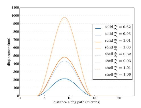
FIGURE A.2: Effect of the element's type (solid or shell elements) on the elastic-plastic buckling of straight blister. The profiles obtained are given for different  $\sigma_0$  and the same hardening law (Ludwik  $\sigma_y = 800 \text{ MPa}$ , K = 130 MPa, n = 0.25)
