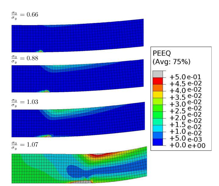
FIGURE 3.6: Equivalent plastic strain mapping for the cases  $\frac{\sigma_0}{\sigma_y}=0.66$ ,  $\frac{\sigma_0}{\sigma_y}=0.88$  and  $\frac{\sigma_0}{\sigma_y}=1.03$ . All cases are subject to the same residual stresses ( $\sigma_0=800~\mathrm{MPa}$ ). The elastic-plastic behaviour is described by Ludwik hardening with the following fixed parameters  $K=130~\mathrm{MPa}$ , n=0.25. We vary  $\sigma_y$
