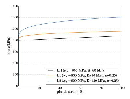
FIGURE 3.14: Stress as a function of plastic strain for Linear plasticity and Ludwik laws
