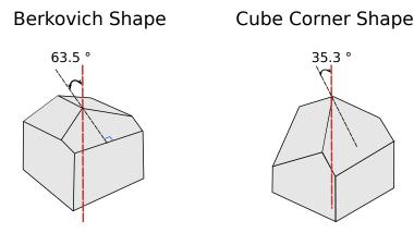
FIGURE 2.5: Berkovich and cube corner indenter tip geometries
