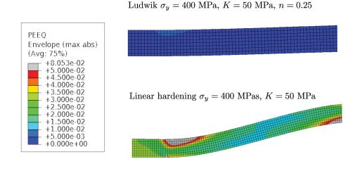
FIGURE 3.17: Effect of the hardening law on plastic strain at the base of straight blisters ( $\sigma_0 = 404$  MPa)
