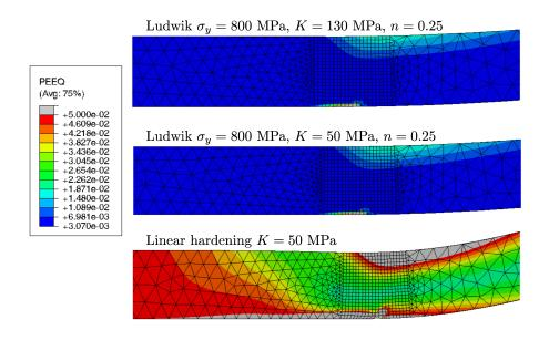
FIGURE 3.16: Effect of the hardening law on plastic strain at the base of straight blisters ( $\sigma_0 = 802 \text{ MPa}$ )
