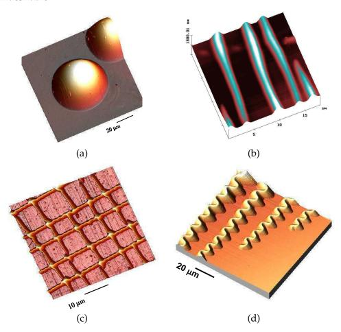
FIGURE 1: Examples of buckling delamination structures. (a) Circular blisters – Au(630 nm) on Si. (b) Straight sided blisters – stainless steel. (c) Intersecting blisters – Stainless steel on polycarbonate. (d) Telephone cords blisters –  $Y_2O_3(30\text{-}50\text{nm})$  on GaAs. (Courtesy of C. Coupeau et col., Institut P')
