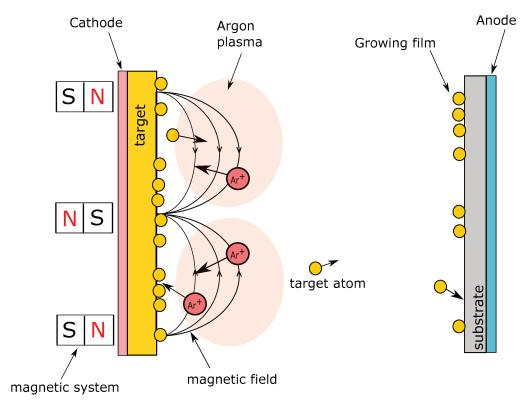
FIGURE 2.1: Scheme of magnetron sputtering device
