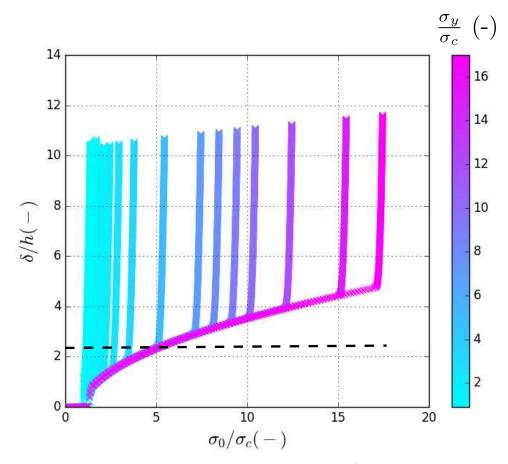
FIGURE 3.12: 2D projection of normalized deflection  $\frac{\delta}{h}$  as function of  $\frac{\sigma_0}{\sigma_c}$ . The graph features different level lines of  $\frac{\sigma_y}{\sigma_c}$ . These curve are plotted for a Ludwik hardening:  $K=130~\mathrm{MPa}$  and n=0.25.
