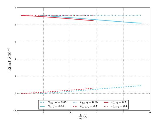
FIGURE 4.6: Energy as a function of the normalized position of the crack front  $\frac{b}{b_0}$ , where b is the half width of the blister and  $b_0$  the half width of the initial defect.  $E_e$  represents the elastic energy and  $E_{sep}$  the energy used to fracture the interface.
