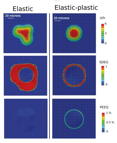
FIGURE 4.28: Various stages of growth of a circular blister submitted to constant load  $\sigma_0$  in the case of an elastic and an elastic-plastic behaviour ( $\sigma_y = 800 \text{ MPa}, K = 50 \text{ MPa}, n = 0.25$ ). Each case features the mapping of the normalized out-of-plane displacement  $\frac{U}{h}$  at the equilibrium point, the corresponding degradation variable of the interface SGEG and the distribution of the plastic deformation.
