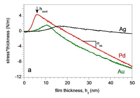
FIGURE 3.20: Film force evolution during sputter deposition of Ag, Au and Pd films on a-SiOx. The film thickness corresponding to the tensile peak is referred as  $h_{cont}$
