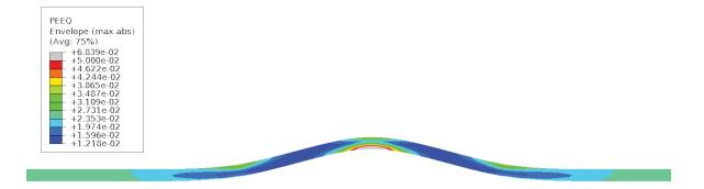
FIGURE 4.17: Equivalent plastic deformation mapping in the cases  $\sigma_0 = 420$ . The remaining parameters are detailed in table 4.5.
