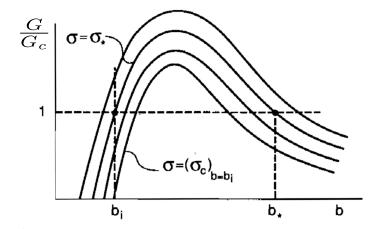
FIGURE 1.15: , Evolution of the ratio  $\frac{G}{G_c}$  during straight blister's propagation based on mode mixity dependent toughness, from [48]
