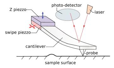
FIGURE 2.2: Scheme of an atomic force microscope
