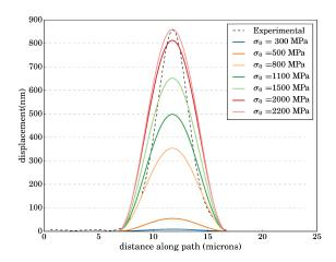
FIGURE 3.4: Comparison between the experimental profiles of circular (left) and straight (right) buckles with results of FEM simulations assuming a linear elastic behavior of the film, obtained for several values of  $\sigma_0$ .
