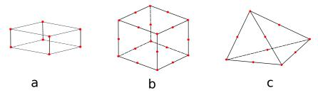
FIGURE A.1: Shell and solid elements: (a) Continuum shell linear elements (8-node brick, SC8R), (b) Solid quadratic element (20-node brick, C3D20), (c) Solid quadratic element (10-node tetrahedron, C3D10)
