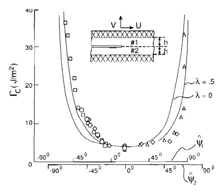
FIGURE 1.8: Data from [65] for an epoxy \$1 / glass \$2 interface:  $\psi_1$  axis is obtained using  $l_1 = 12,7mm$  and  $\psi_2$  using  $l_2 = 127\mu m$ . The solid curves represent  $G_c(\psi_2)$  as given by equation 1.35
