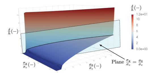
FIGURE 3.11: 3D representation of the normalized deflection  $\frac{\delta}{h}$  as function of  $\frac{\sigma_y}{\sigma_c}$  and  $\frac{\sigma_0}{\sigma_c}$ . This curve is plotted using the following Ludwik hardening:  $K=130~\mathrm{MPa}$  and n=0.25.
