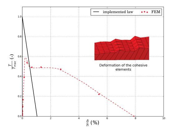
FIGURE 4.9: This graph features the implemented cohesive law and the corresponding cohesive response obtained via FEM implicit analysis with a time step  $\tau=0.1$  and a viscous relaxation time of  $\mu=1.e-4$ . The graph also shows the state of cohesive elements in contact with the distorted 3D elements showed in figure 4.8.
