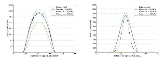
FIGURE 3.25: Effect of non-monotonic loading on elastic-plastic buckling in the case of circular blister (left  $\sigma_y=800~\mathrm{MPa}$ ) and straight blister (right  $\sigma_y=400~\mathrm{MPa}$ ) (Ludwik strain hardening  $K=50~\mathrm{MPa}$ , n=0.25)
