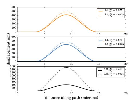
FIGURE 3.15: Straight blisters' profiles for different elastic-plastic behaviours: L1 (Ludwik: $\sigma_y = 800 \text{ MPa}$ , K = 50 MPa, K = 0.25), L2: (Ludwik:K = 0.25), L2: (Ludwik:K = 0.25), LH (Linear hardening:K = 0.25), LH (Linear hardening:K = 0.25)
