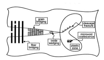
FIGURE 1.10: Schematic illustration of several physical mechanisms occurring in materials during crack growth. from [86]
