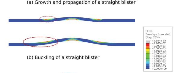
FIGURE 4.13: Equivalent plastic deformation mapping in the cases of pure buckling (a) and buckling-driven delamination (b). Both results were obtained for the same load and elastic plastic behaviour. We have  $\sigma_0 = \sigma_y = 700$ . The remaining parameters are detailed in table 4.4.
