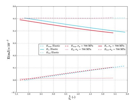
FIGURE 4.14: Energy as a function of the normalized position of the crack front  $\frac{b}{b_0}$ , where b is the half width of the blister during propagation and  $b_0$  the half width of the initial defect.  $E_e$  represents the elastic energy,  $E_p$  the plastic energy and  $E_{sep}$  the energy used to fracture the interface. The figure feature two cases: purely elastic thin film ( $\sigma_0 = 700 \text{ MPa}$ ) and elastic-plastic thin film ( $\sigma_0 = \sigma_y = 700 \text{ MPa}$ ).
