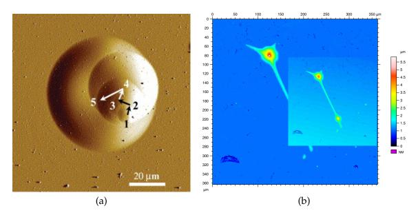
FIGURE 4.31: Examples of unresolved cases of buckling delamination structures in gold thin film. (a) Signal error-mode atomic force microscopy image of a snail like blister. The rings result from the successive growth of one circular blister in a gold thin film, labelled from initial state 1 to the final position 5. – Au(630 nm) on Si [18]. (b) interaction between straight and circular blisters – Au(200 nm) on Si.(Courtesy of C. Coupeau, Institut P')
