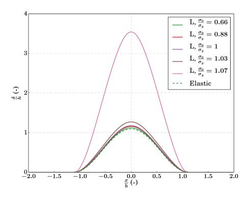
Figure 3.5: Comparison between elastic and elastic-plastic straight blisters' profiles. The y-axes represents normalized deflection  $\frac{\delta}{h}$ , where  $\delta$  is the out-of-plane displacement of the film and h the thickness of the film (fixed). All cases are subject to the same residual stresses ( $\sigma_0 = 800 \text{ MPa}$ ). The elastic-plastic behaviour is described by Ludwik hardening with the following fixed parameters K = 130 MPa, n = 0.25. We vary  $\sigma_y$
