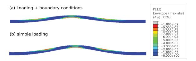
FIGURE 4.24: Mapping of equivalent plastic deformation. (a) Results obtained by blocking the displacement of the nodes at the bottom of the defect area during the loading. (b) Results obtained using simple loading with no restrictions on the displacement of certain parts of the film.
