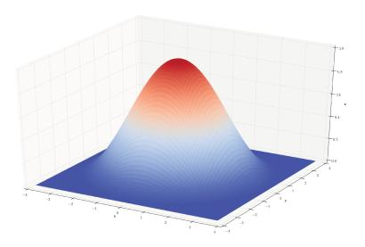
FIGURE 1.3: Representation of the analytical solution  $w_1(\rho)$ . The X-, Y-, and Z-axis origin point has been set at the centre of the bubble's basis.
