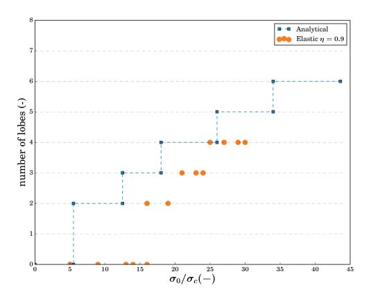
FIGURE 4.26: Number of lobes n resulting from the destabilization process of an initially circular blister at different loading ratios  $\frac{\sigma_0}{\sigma_c}$ . Numerical results are obtained using cohesive zone model for a mode mixity dependence parameter  $\eta=0.9$  and Poisson's ratio of the film  $\nu=0.44$ . The analytical results are obtained for  $\eta=1$  and  $\nu=\frac{1}{3}$ .
