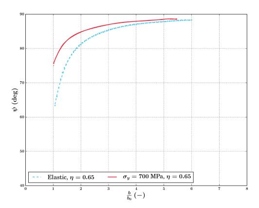
FIGURE 4.15: Mode mixity angle  $\psi$  as a function of the normalized position of the crack front  $\frac{b}{b_0}$ , where b is the half width of the blister and  $b_0$  the half width of the initial defect in the case of an elastic and an elastic-plastic response of the film.
