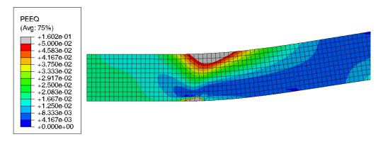
FIGURE 3.9: Equivalent plastic mapping of the case ( $\frac{\sigma_0}{\sigma_c} = 0.5$ ,  $\frac{\sigma_0}{\sigma_u} = 1.05$ )
