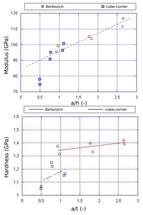
FIGURE 2.8: Indentation modulus and hardness as function of normalized equivalent contact radius  $\frac{a}{t}$  for 400 nm gold thin film deposited on silicon substrate. The red circles correspond to Berkovich indenter data while the blue squares correspond to cube-corner indenter data.
