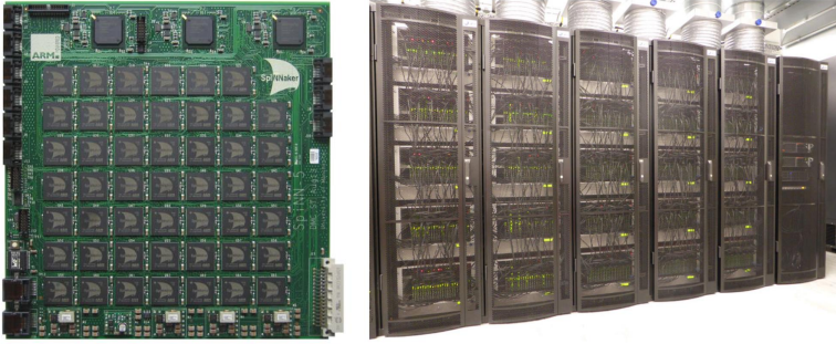
Figure 13: Left: Circuit board of the SpiNNaker device composed of ARM processors. Right: The 500 000 cores SpinNNaker Human Brain platform. Extracted from Hopkins et al. [1].
